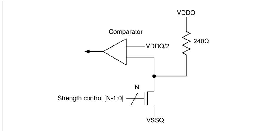
**Figure 164 - Pull-down calibration**
