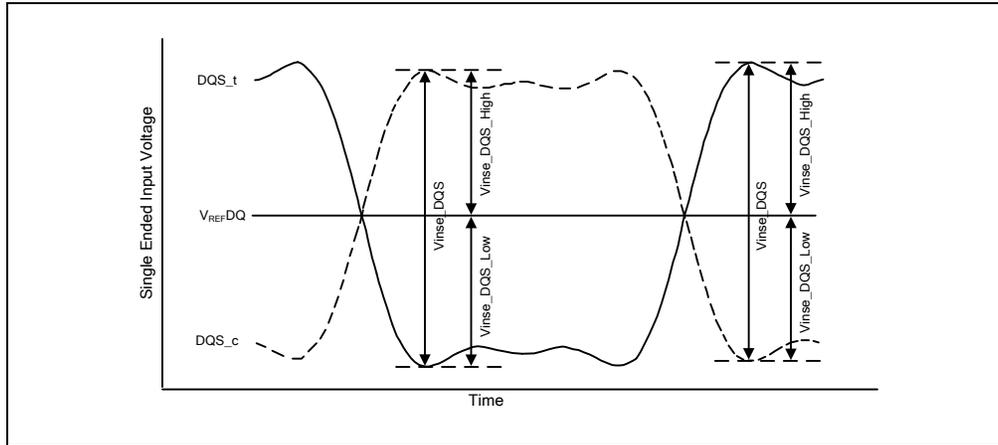
**Note:** 1.  $V_{REFDQ}$  is LPDDR4X SDRAM internal setting value by  $V_{REF}$  Training.
