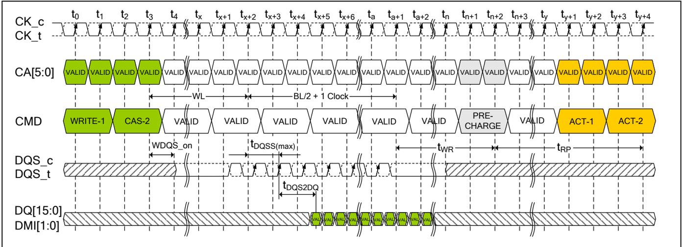
Figure 58 - Burst WRITE Followed by PRECHARGE
