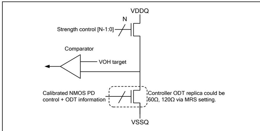
**Figure 165 - Pull-up calibration**
