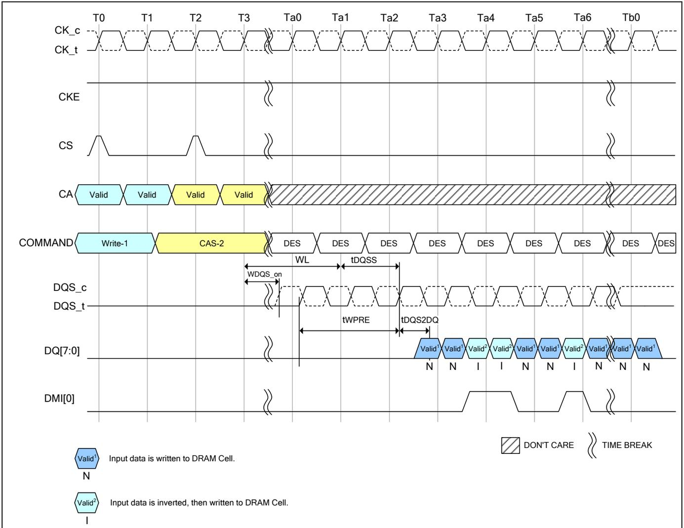
**Note:** 1. Data Mask (DM) is Disable: MR13 OP[5] = 1, Data Bus Inversion (DBI) Write is Enable: MR3 OP[7] = 1.
