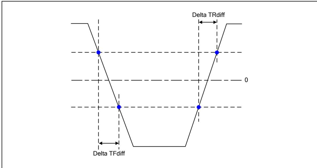
Figure 160 - Differential Output Slew Rate Definition
