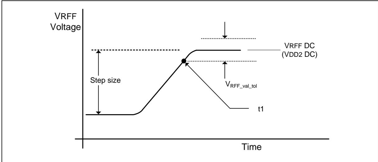
Figure 87 - VREF step single step size increment case
