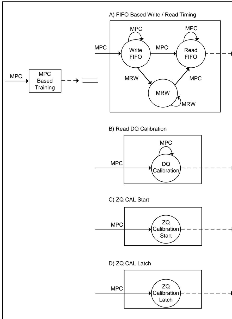
**Figure 2 - Simplified Bus Interface State Diagram-2**
