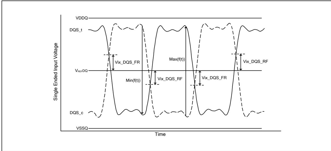
**Note:** 1. The base level of V<sub>ix\_DQS\_FR/RF</sub> is V<sub>REFDQ</sub> that is LPDDR4X SDRAM internal setting value by V<sub>REF</sub> Training.
