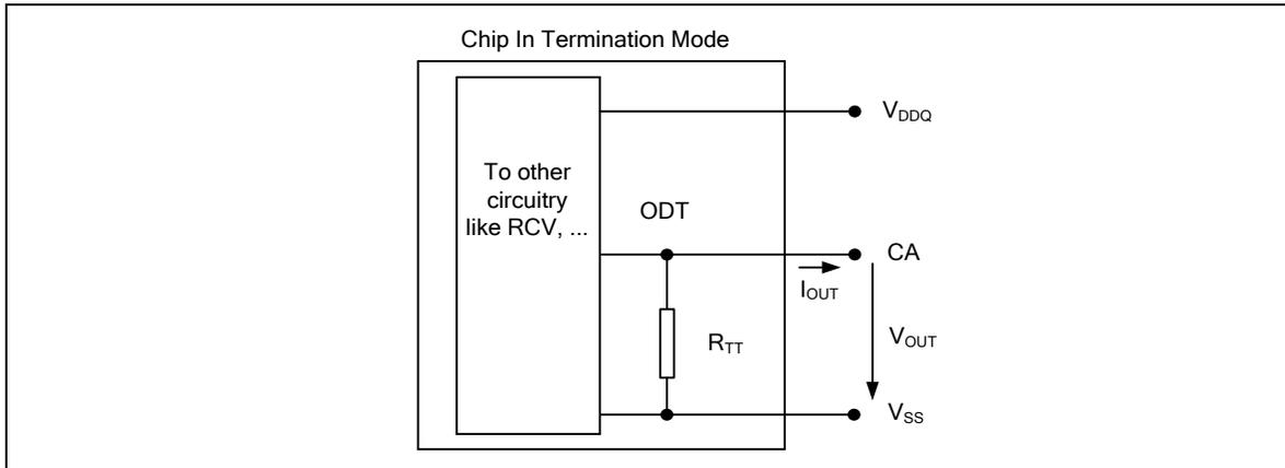
Figure 128 - On Die Termination for CA
