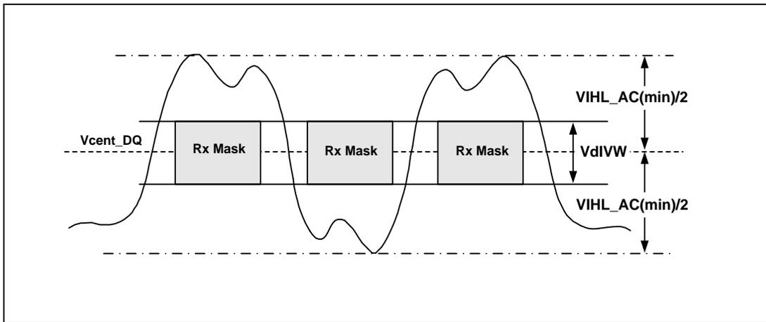
**Figure 177 - DQ VIH\_L\_AC definition (for each input pulse)**
