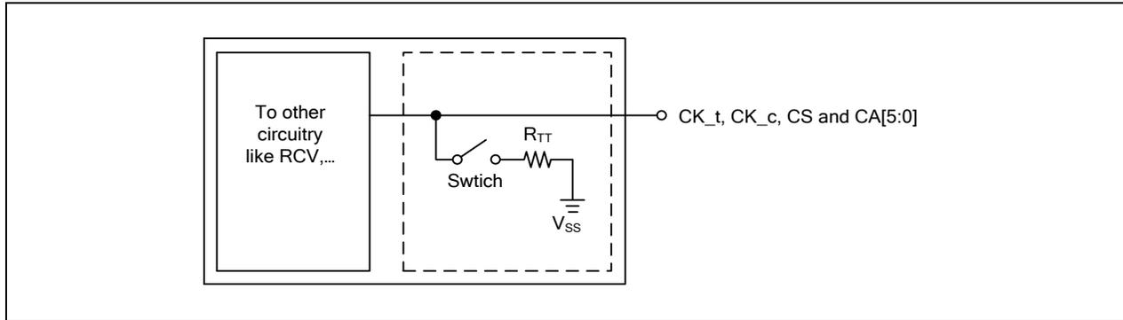
Figure 127 - Functional Representation of CA ODT
