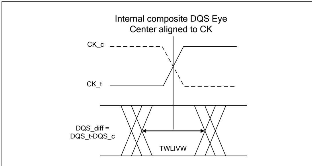
Figure 109 - DQS<sub>t</sub>/DQS<sub>c</sub> to CK<sub>t</sub>/CK<sub>c</sub> timings at the DRAM pins referenced from the internal latch
