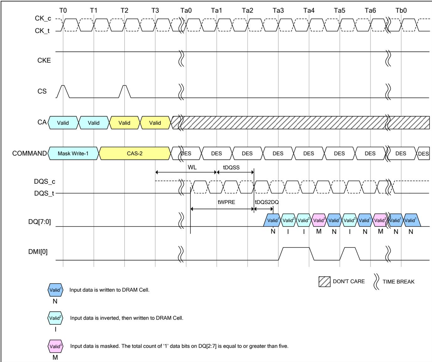
Note: 1. Data Mask (DM) is Enable: MR13 OP[5] = 0, Data Bus Inversion (DBI) Write is Enable: MR3 OP[7] = 1.
