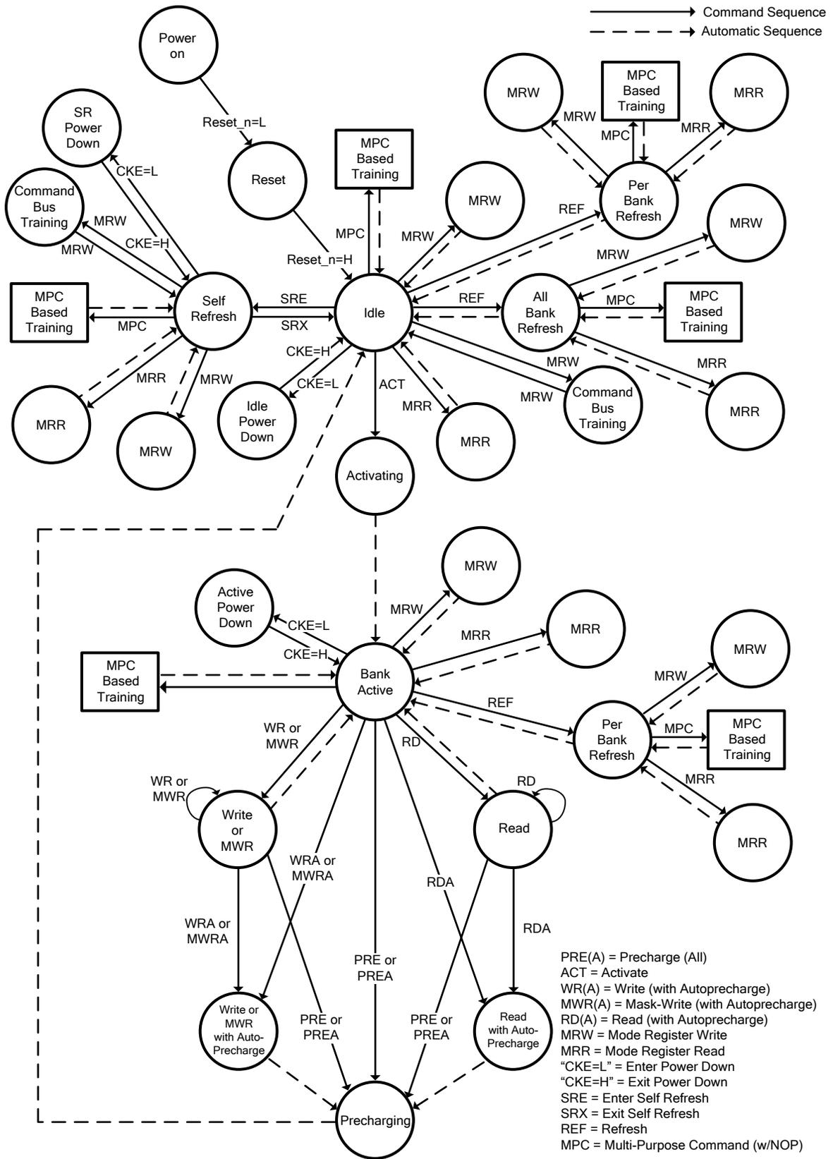
Figure 1 - Simplified Bus Interface State Diagram-1
