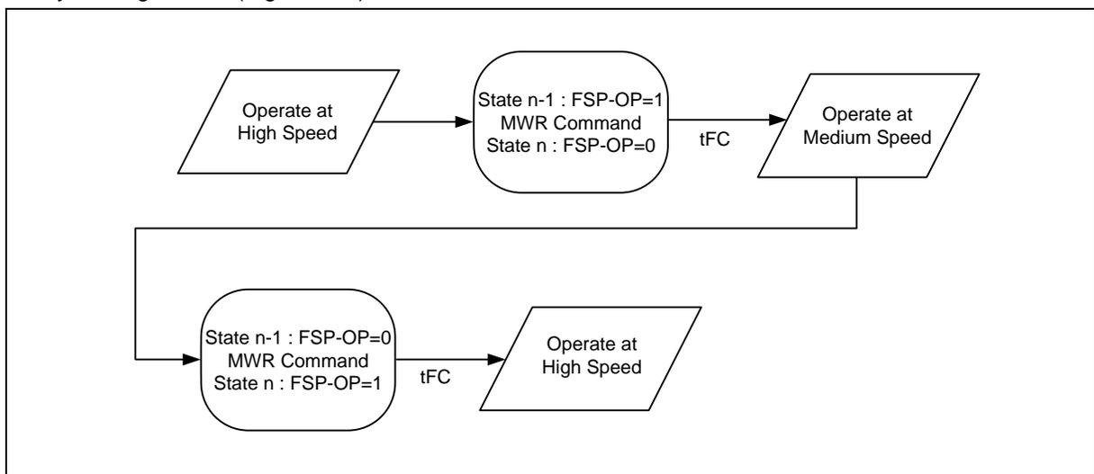
Figure 104 - Switching Between Two Trained Frequency Set-Points
