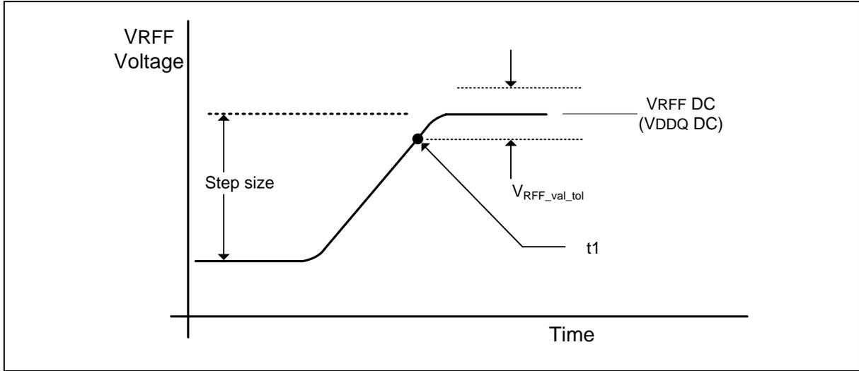
Figure 94 - VREF step single step size increment case
