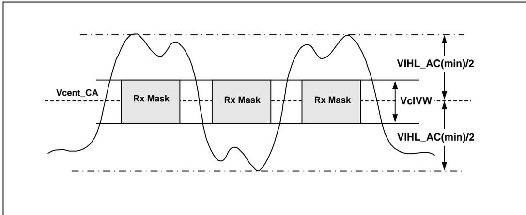
Figure 170 - CA VIH<sub>L</sub>\_AC definition (for each input pulse)
