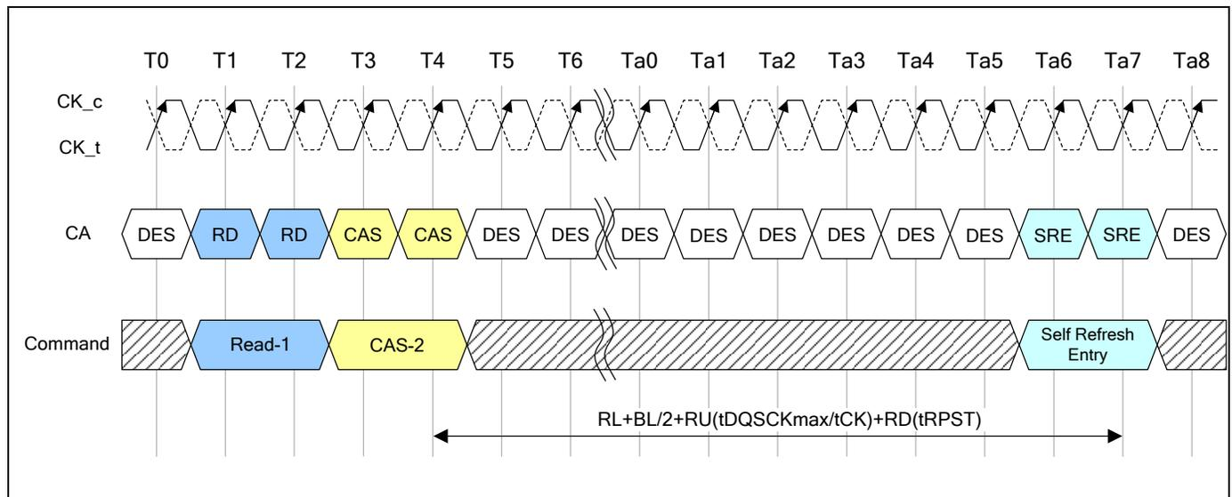
During Self Refresh mode, external clock input is needed and all input pin of SDRAM are activated. SDRAM can accept the following commands, MRR-1, CAS-2, DES, SRX, MPC, MRW-1, and MRW-2 except PASR Bank/Segment setting.
