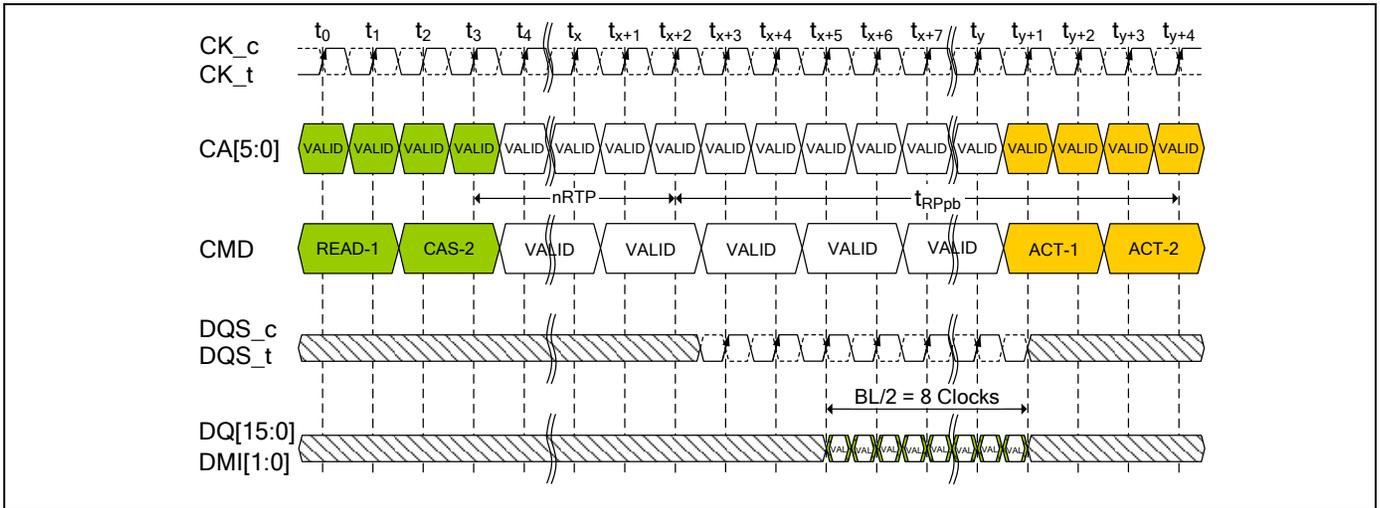
**Figure 59 - Burst READ with Auto-Precharge
