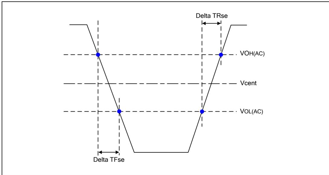
Figure 159 - Single Ended Output Slew Rate Definition
