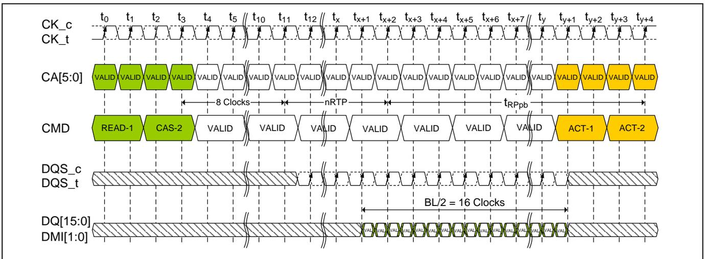
**Figure 60 - Burst READ with Auto-Precharge
