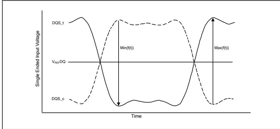
**Note:** 1.  $V_{REFDQ}$  is LPDDR4X SDRAM internal setting value by  $V_{REF}$  Training.
