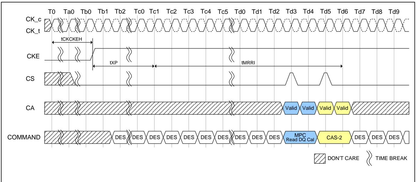
Figure 112 - MPC Read DQ Calibration Following Power-Down State
