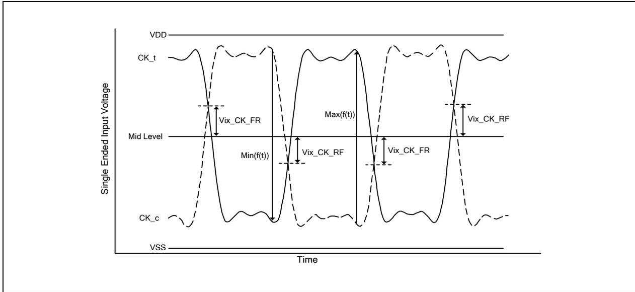
**Note:** 1. The base level of Vix\_CK\_FR/RF is V<sub>REFCA</sub> that is LPDDR4X SDRAM internal setting value by V<sub>REF</sub> Training.
