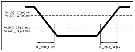
Figure of Input C Slew Rate Definition
