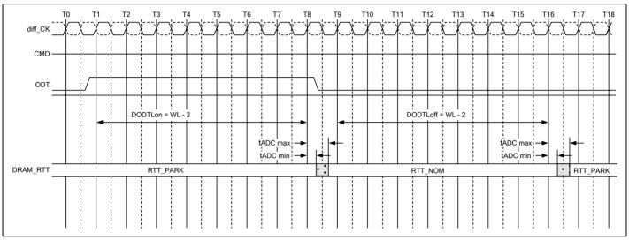
Figure 163 – Synchronous ODT Timing Example for CWL=9, AL=0, PL=0; DODTLon=WL-2=7; DODTLoff=WL-2=7
