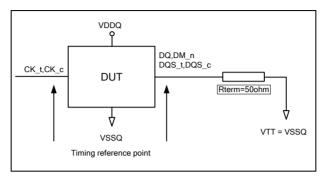
Figure 172 - ODT Timing Reference Load
