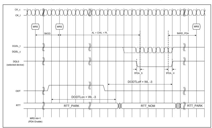
Note: RTT PARK = Enable, RTT NOM = Enable, Write Preamble Set = 2tck and DLL = ON, CA parity is used
