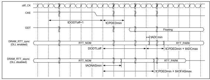
Figure 170 - ODT timing for power down entry with ODT buffer disable mode
