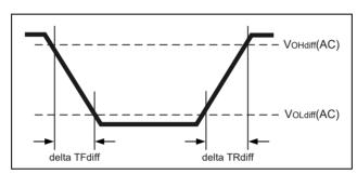
Figure 192 - Differential Output Slew Rate Definition
