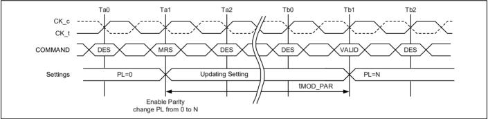
Figure 48 - Parity entry timing example - tMRD\_PAR
