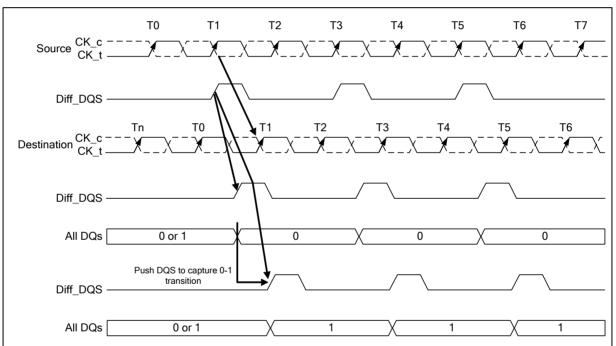
Figure 9 - Write Leveling Concept
