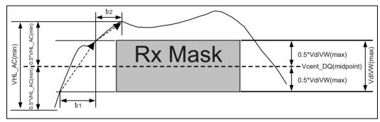
Figure 201 - Slew Rate Conditions for Rising Transition
