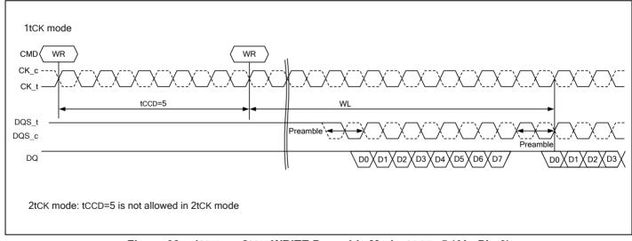
Figure 62 – 1tCK vs. 2tCK WRITE Preamble Mode, tCCD=5 (AL=PL=0)
