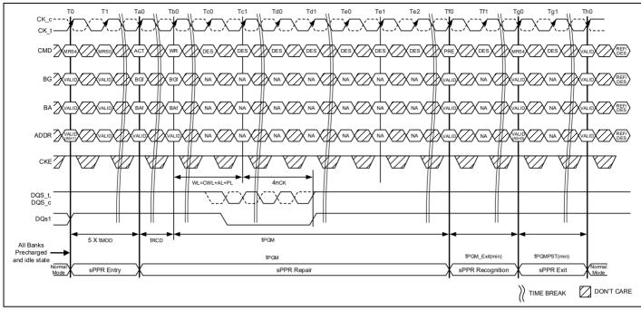
Figure 160 - Fail Row Soft PPR (WR Case)
