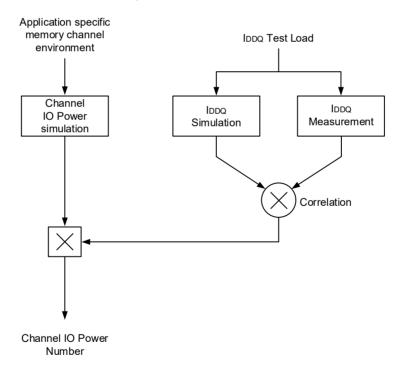
Figure 196 – Correlation from simulated Channel IO Power to actual Channel IO Power supported by IDDQ Measurement
