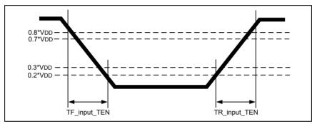
Figure 155 - TEN Input Slew Rate Definition
