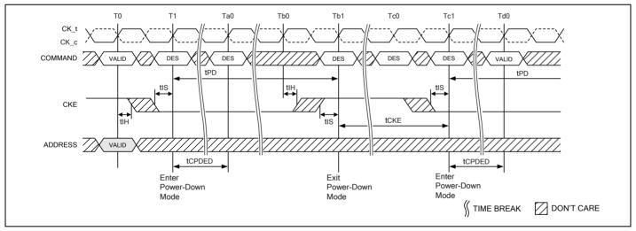
Figure 152 - Power-Down Entry/Exit Clarification
