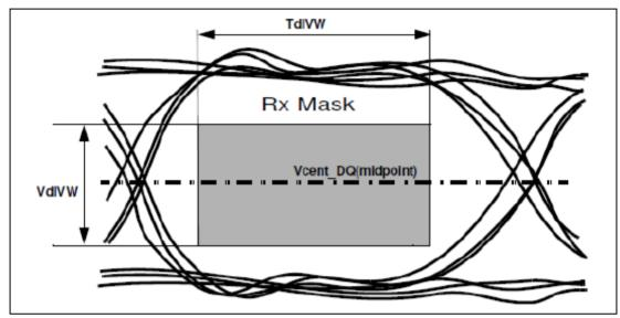
Figure 198 - DQ Receiver (Rx) compliance mask
