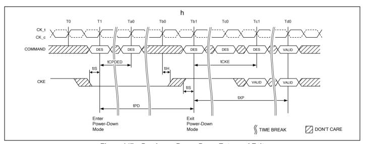
Figure 147 - Precharge Power-Down Entry and Exit
