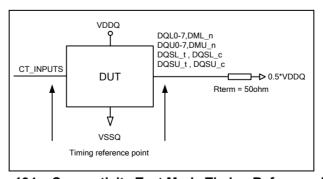
Figure 194 – Connectivity Test Mode Timing Reference Load
