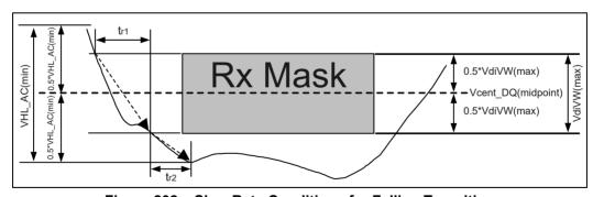
Figure 202 – Slew Rate Conditions for Falling Transition
