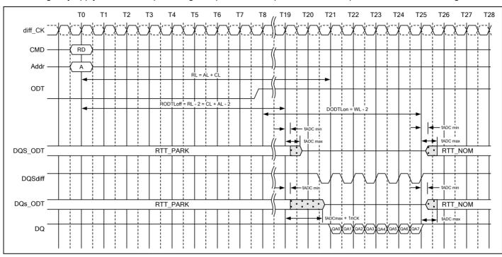
Figure 165 – Example: CL=11, PL=0; AL=CL-1=10; RL=AL+PL+CL=21; CWL=9; DODTLon=AL+CWL-2=17; RODTLoff=CL+AL-2=19; 1tCK preamble
