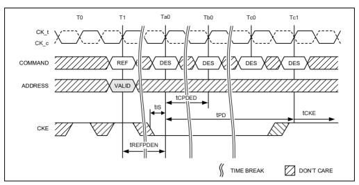
Figure 148 - Refresh Command to Power-Down Entry
