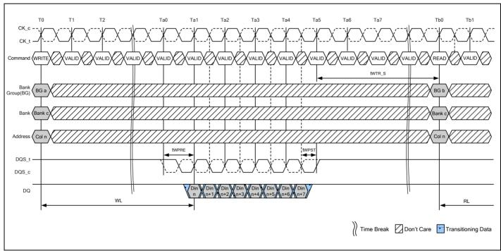
Note: tWTR\_S: Delay from start of internal write transaction to internal read command to a different Bank Group. When AL is non-zero, the external read command at Tb0 can be pulled in by AL.
