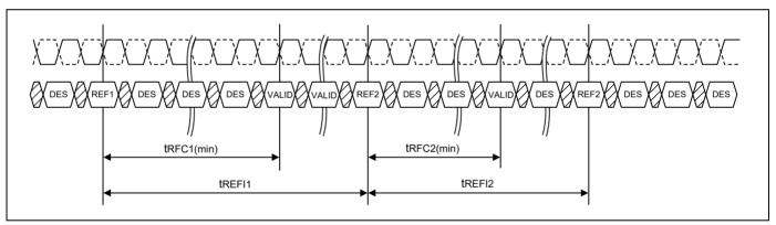
Figure 12 - On-the-fly Refresh Command Timing
