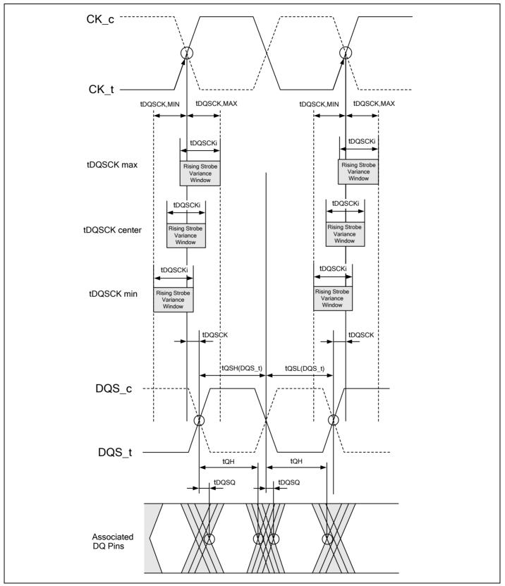
Figure 64 - READ Timing Definition
