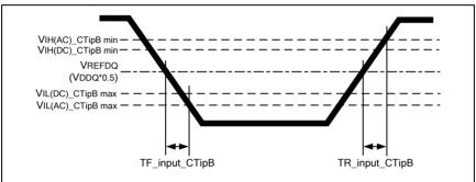
Figure 157 - Input B Slew Rate Definition
