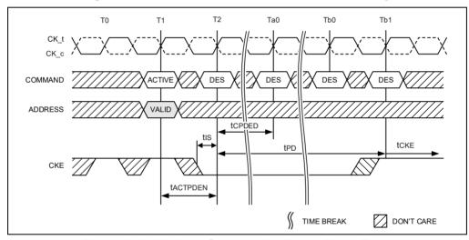
Figure 149 - Activate Command to Power-Down Entry
