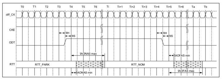
Figure 169 – Asynchronous ODT Timing on DDR4 SDRAM with DLL-off
