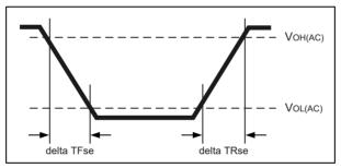
Figure 191 - S ingle-ended Output Slew Rate Definition
