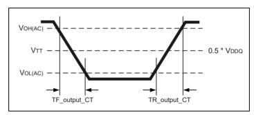
Figure 193 – Output Slew Rate Definition of Connectivity Test Mode
