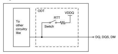
Figure 161 - Functional Representation of ODT
