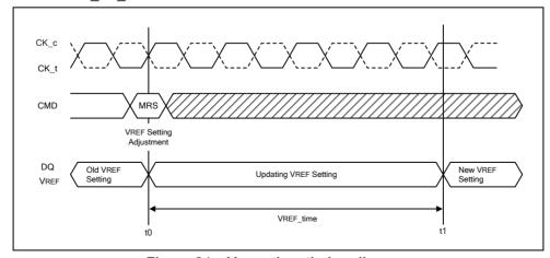
Figure 24 – VREF\_time timing diagram
