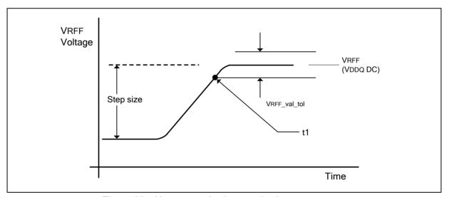
Figure 26 - VREF step single step size increment case
