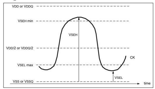
Figure 178 - Single-ended requirement for differential signals
