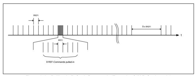
Figure 140 – Pulling-in Refresh Commands (Example of 1X Refresh mode)
