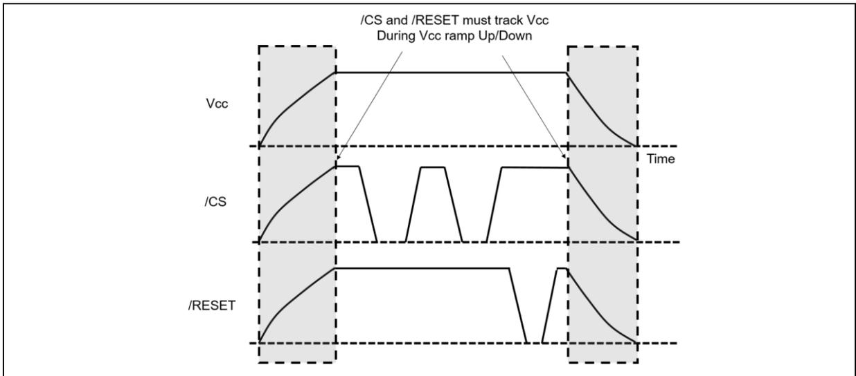
Figure 9-2 Power-up, Power-down Requirement
