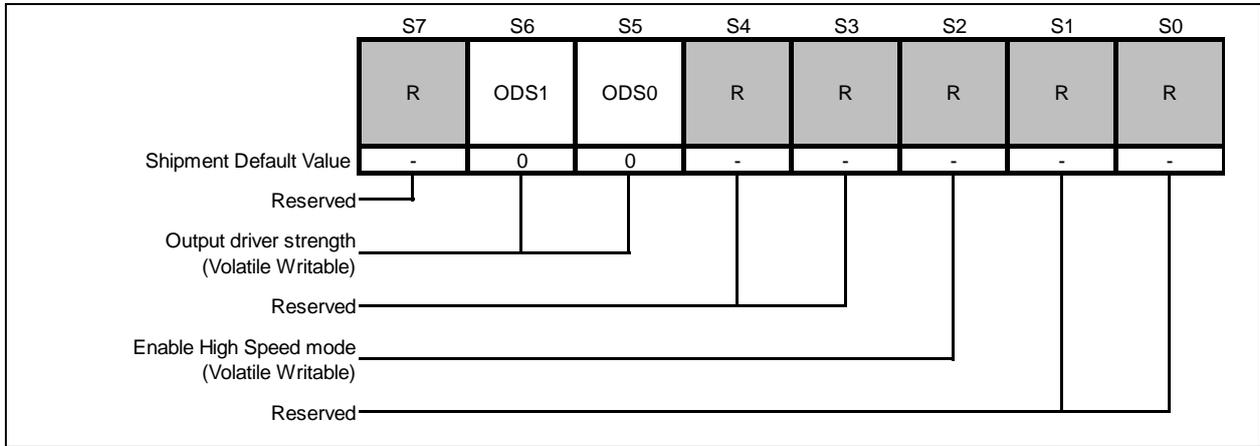
Figure 7-4 Status Register-4 (Address D4h)
