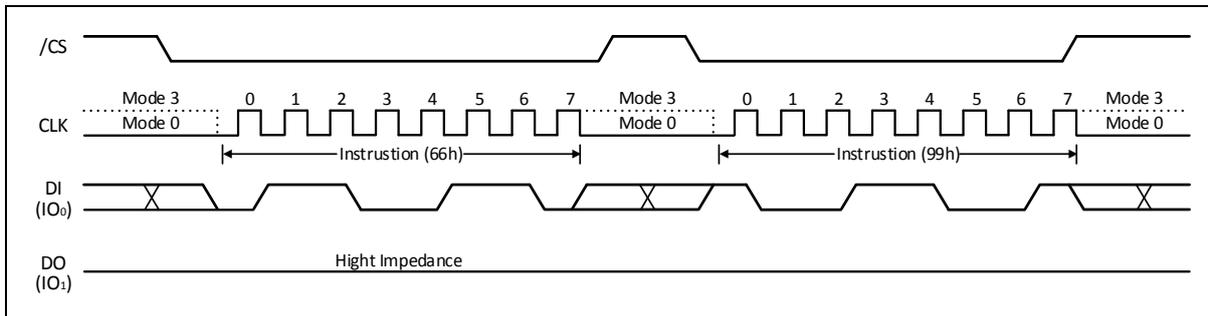
Figure 8-2 Device Reset Instruction (66h+99h)
