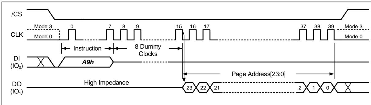
Figure 8-10 Last ECC Failure Page Address Instruction
