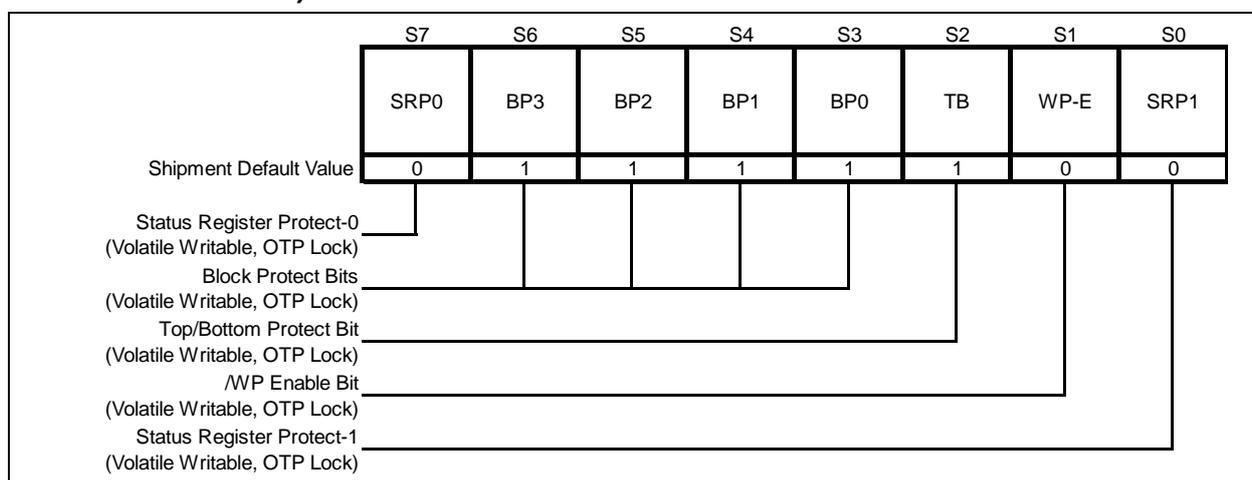
Figure 7-1 Protection Register / Status Register-1 (Address Axh)
