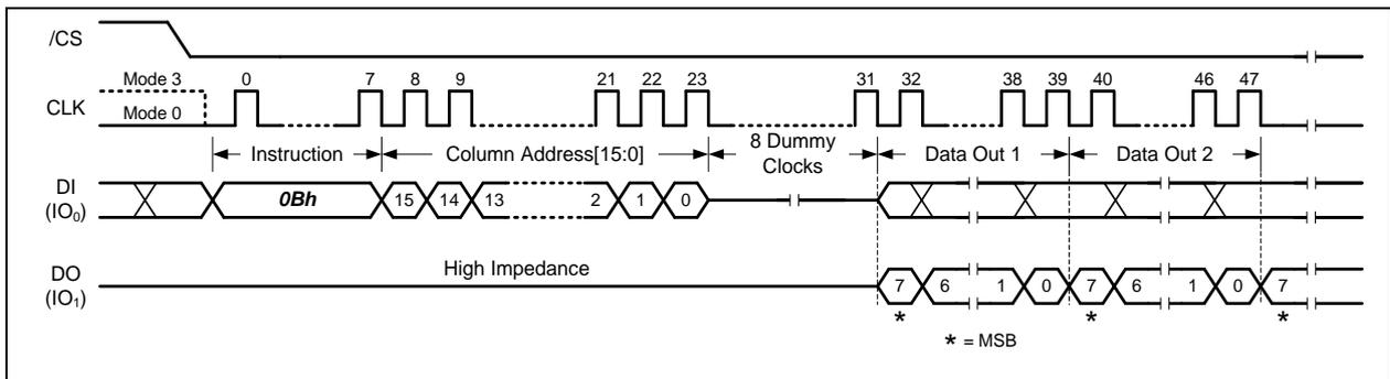
Figure 8-23 Fast Read Instruction (Buffer Read Mode, BUF=1)
