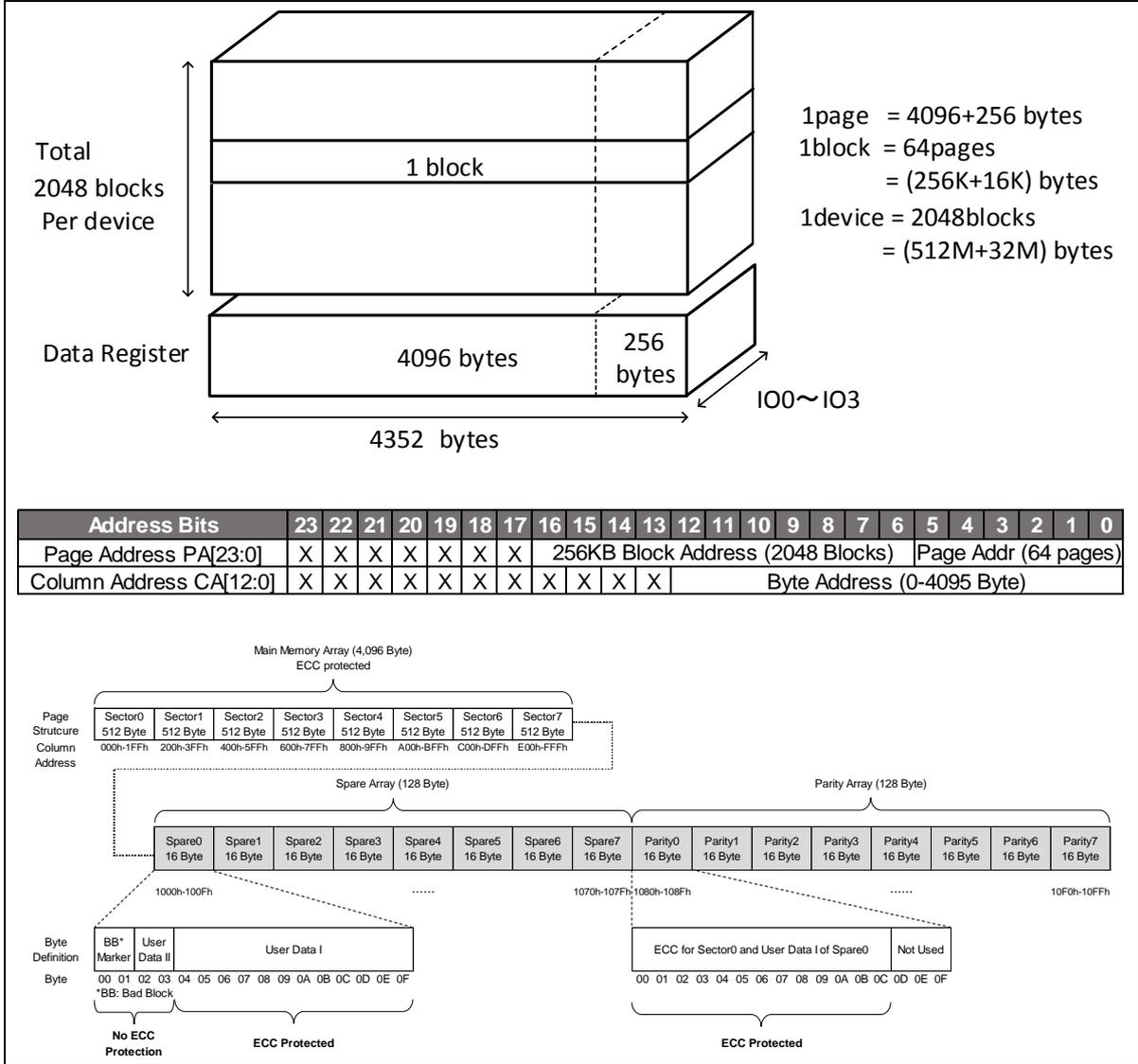
Figure 5-1 W25N04LW Flash Memory Architecture and Addressing
