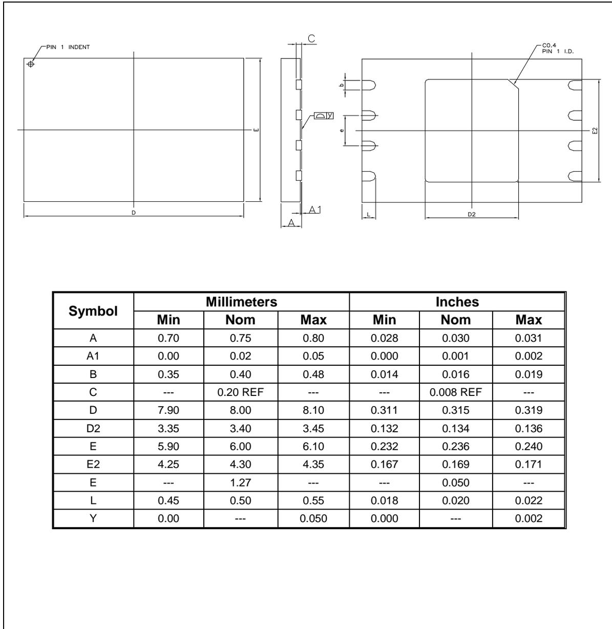
Figure 11-1 8-Pad WSON 8x6-mm (Package Code ZE)
