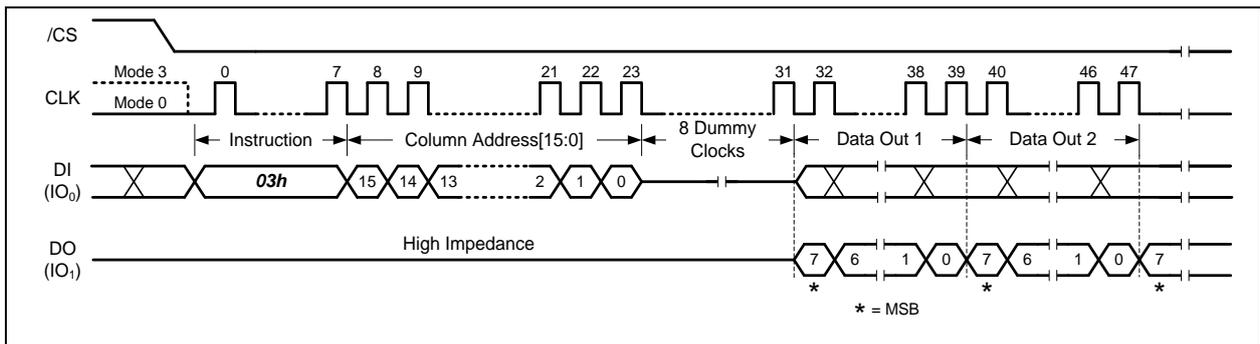
Figure 8-21 Read Data Instruction (Buffer Read Mode, BUF=1)
