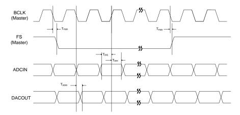
Figure 32: Digital Audio Interface Master Mode Timing
