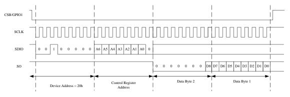
Figure 21: Register Read operation through a 32-bit SPI Interface
