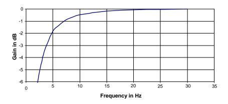
Figure 37: ADC Highpass Filter Response, Audio Mode
