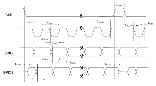
Figure 29: 4-wire Control Mode Timing
