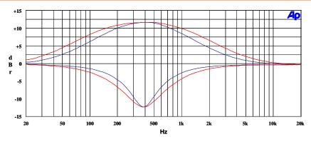
Figure 43: EQ Band 2, EQ2BW = 0 versus EQ2BW = 1
