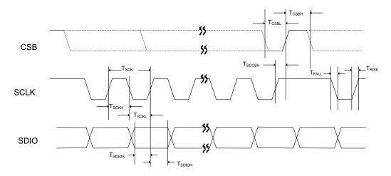
Figure 28: 3-wire Control Mode Timing
