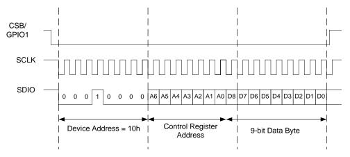
Figure 20: Register Write operation using a 24-bit SPI Interface
