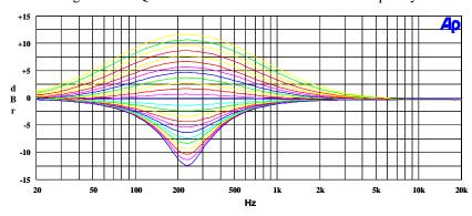
Figure 42: EQ Band 2 Peak Filter Gains for Lowest Cut-Off Frequency with EQ2BW = 0
