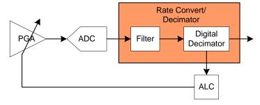
Figure 5: ALC Block Diagram
