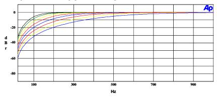
Figure 40: ADC Highpass Filter Response, HPF enabled, FS = 12kHz
