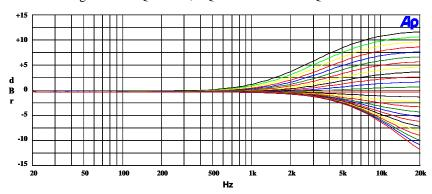
Figure 48: EQ Band 5 Gains for Lowest Cut-Off Frequency
