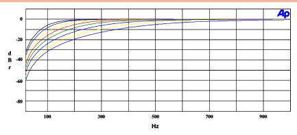
Figure 39: ADC Highpass Filter Response, HPF enabled, FS = 24kHz
