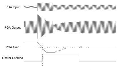
Figure 11: ALC Limiter Mode Operation
