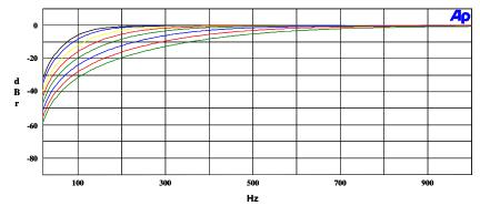
Figure 38: ADC Highpass Filter Response, HPF enabled, FS = 48kHz
