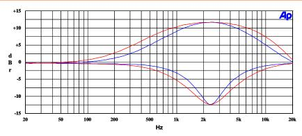
Figure 47: EQ Band 4, EQ4BW = 0 versus EQ4BW =1
