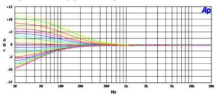
Figure 41: EQ Band 1 Gains for Lowest Cut-Off Frequency
