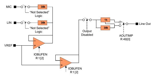
Figure 34: Tie-off Options for input and output pin examples
