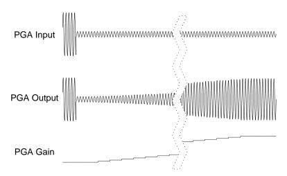
Figure 8: ALC Operation Without Noise Gate
