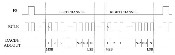
Figure 27: PCM Time Slot Audio Interface
