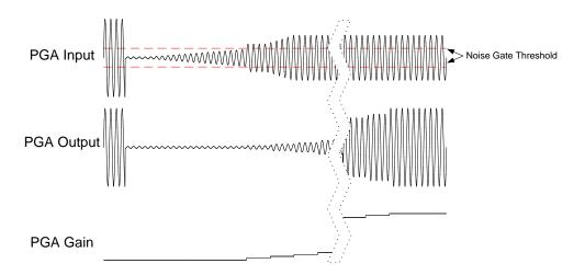
Figure 9: Noise Gate Operation
