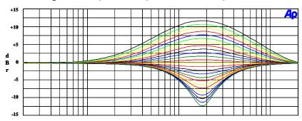
Figure 46: EQ Band 4 Peak Filter Gains for Lowest Cut-Off Frequencies with EQ4BW = 0
