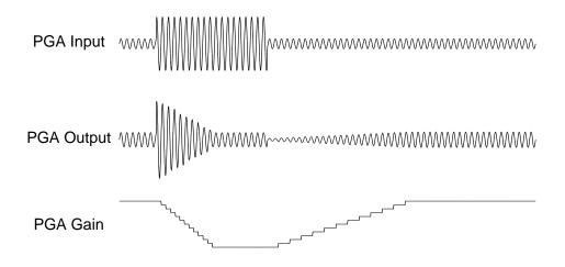
Figure 6: ALC Normal Mode Operation
