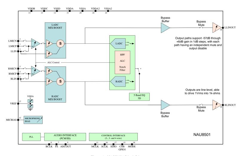
Figure 1: NAU8501 Block Diagram
