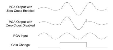
Figure 2: Zero Crossing Gain Update Operation
