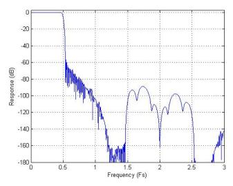
Figure 35: ADC Filter Frequency Response
