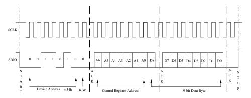
Figure 17: Byte Write Sequence
