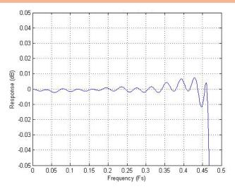
Figure 36: ADC Filter Ripple
