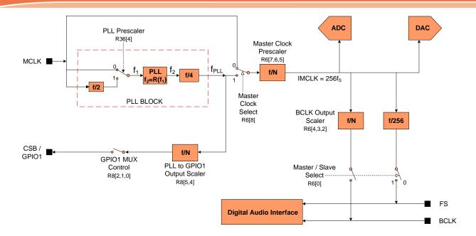
Figure 12: PLL and Clock Select Circuit
