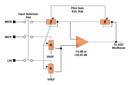
Figure 3: PGA Input Structure Simplified Schematic
