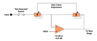
Figure 4: Variable Gain Stage Simplified Schematic
