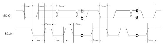
Figure 30: Two-wire Control Mode Timing
