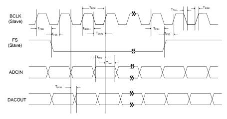
Figure 31: Digital Audio Interface Slave Mode Timing
