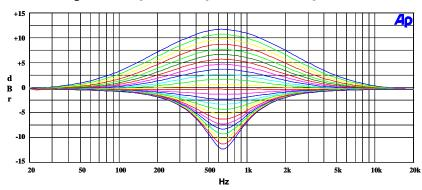
Figure 44: EQ Band 3 Peak Filter Gains for Lowest Cut-Off Frequency with EQ3BW = 0
