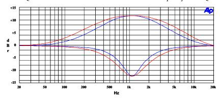
Figure 45: EQ Band 3, EQ3BW = 0 versus EQ3BW = 1
