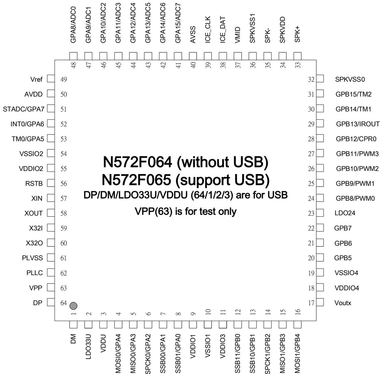
Note1: VPP is for embedded flash test, keep it no connection in general application.
