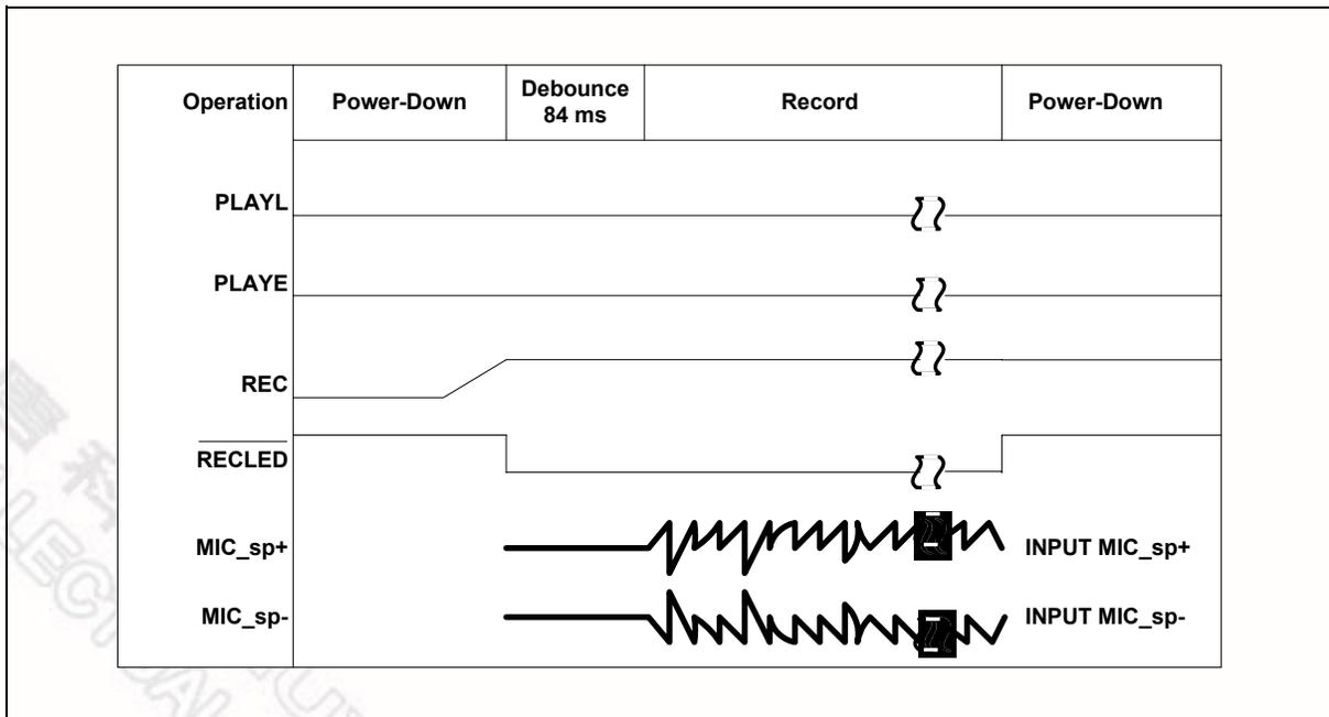
**FIGURE 2: RECORD MESSAGE UNTIL ARRAY IS FULL**
