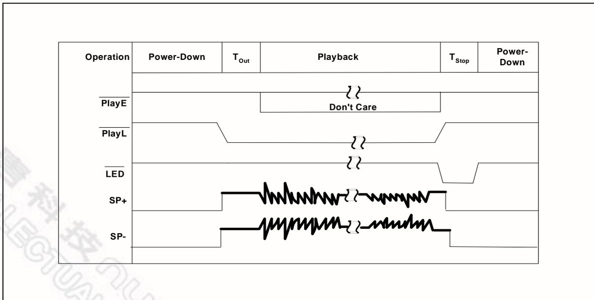
FIGURE 6: LEVEL-TRIGGERED PLAYBACK ( $\overline{\text{PLAYL}}$ ) UNTIL  $\overline{\text{PLAYL}}$  GOES HIGH
