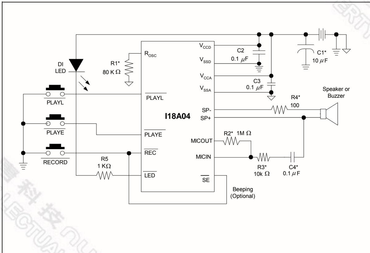
Example #2: Using speaker and microphone separately; recording with LED output
