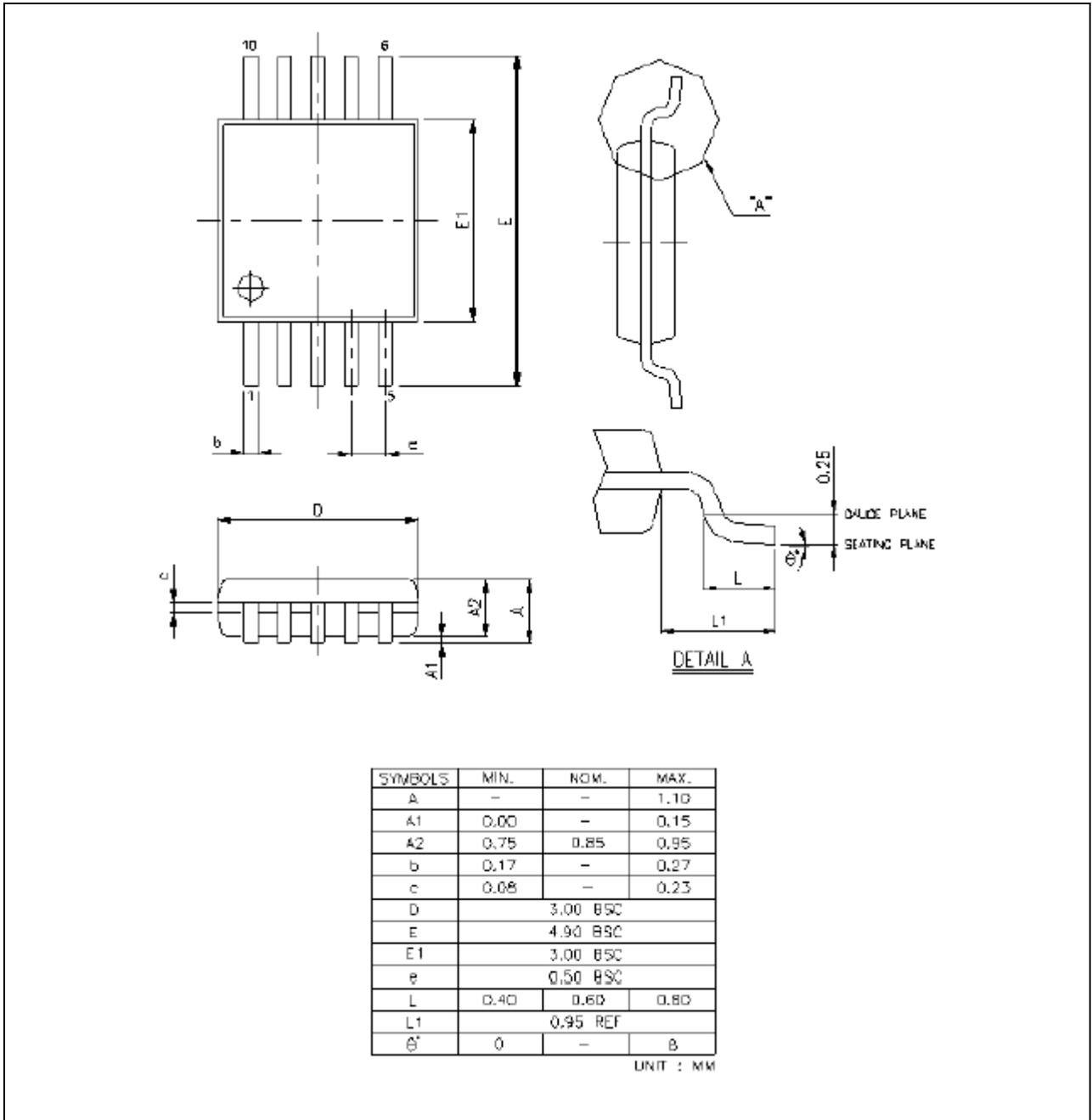
Figure 9.2-1 MSOP -10 Package Dimension
