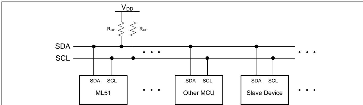
Figure 6.11-1 I<sup>2</sup>C Bus Interconnection
