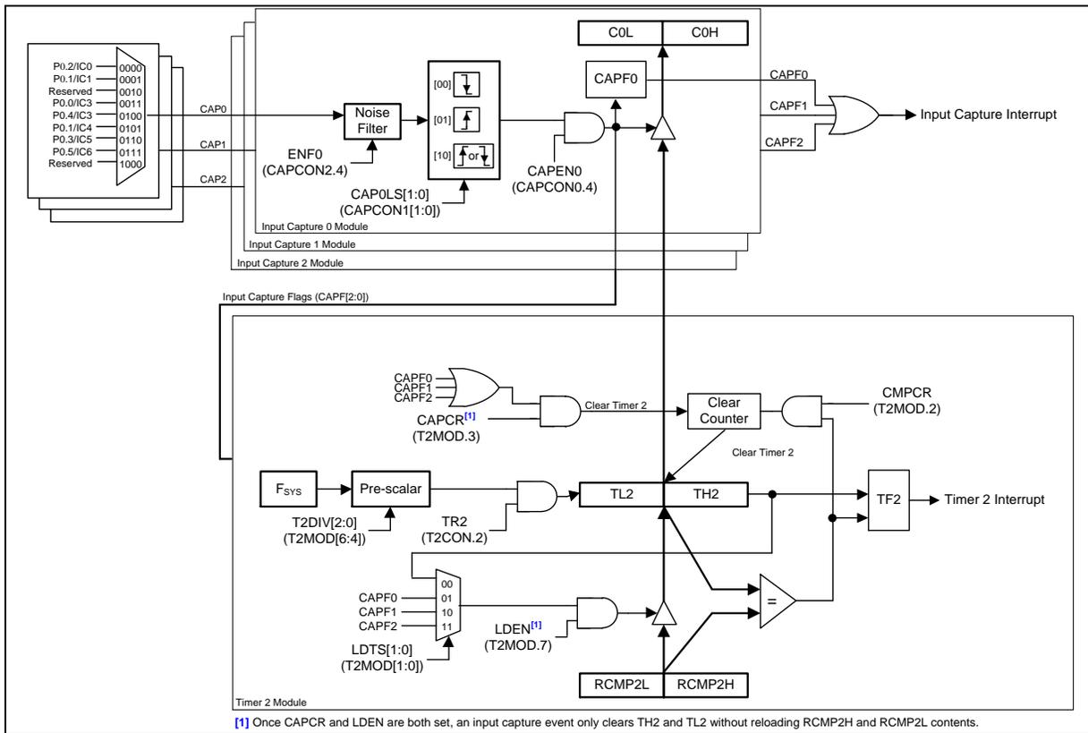
Figure 6.6-1 Timer 2 Full Function Block Diagram
