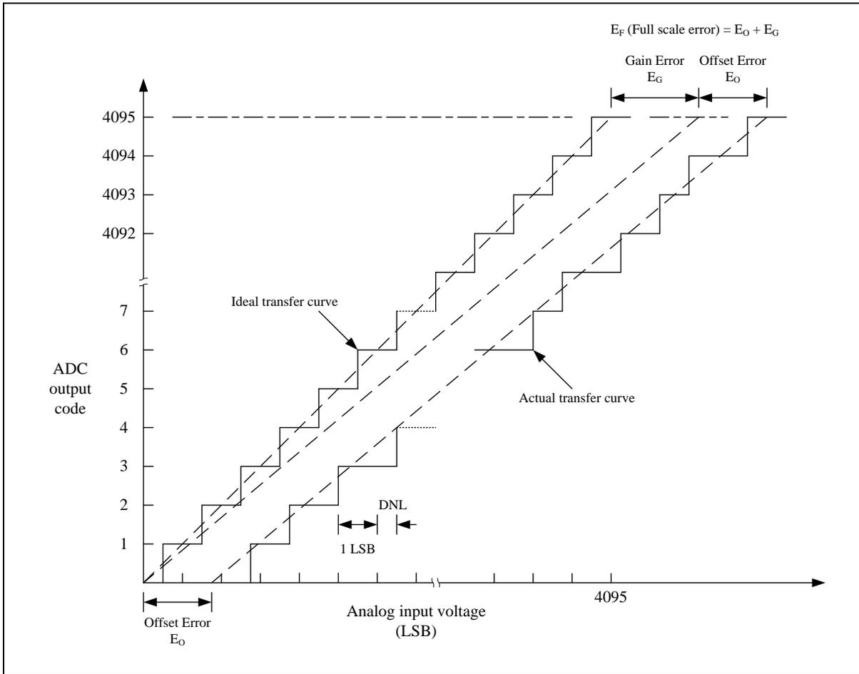
**Note:** The INL is the peak difference between the transition point of the steps of the calibrated transfer curve and the ideal transfer curve. A calibrated transfer curve means it has calibrated the offset and gain error from the actual transfer curve.
