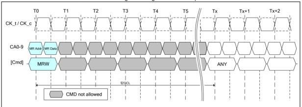
Figure 42 - ZQ Calibration Long Timing
