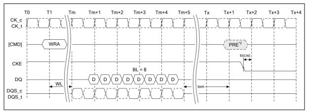
Figure 56 - Write with Auto Precharge to Power-Down Entry
