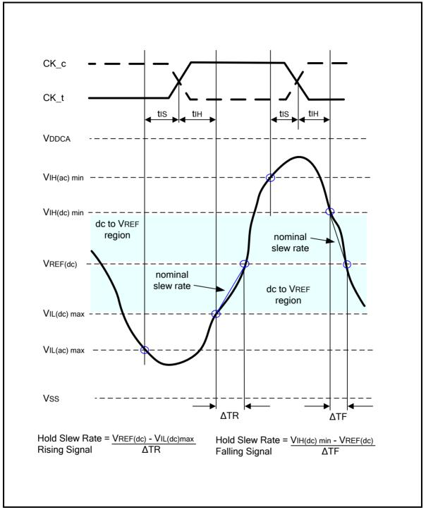
Figure 78 - Nominal slew rate for hold time t<sub>IH</sub> for CA and CS\_n with respect to clock
