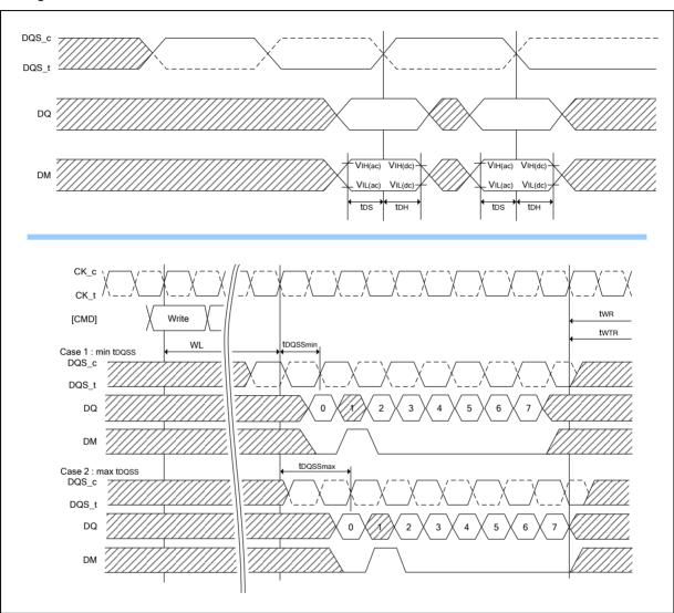
Figure 21 - Data Mask Timing
