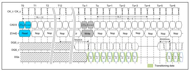
Figure 13 - Burst Read Followed By Burst Write
