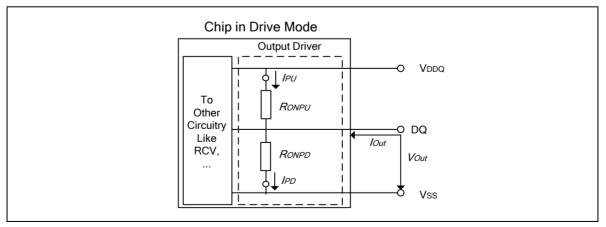
Figure 73 - Output Driver Definition of Voltages and Currents
