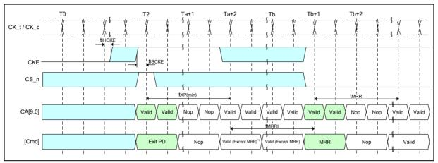
Figure 35 - MRR Following Power-Down Idle State
