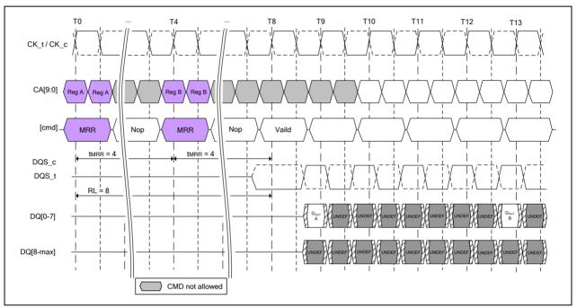
Figure 32 - Mode Register Read timing example: RL = 8
