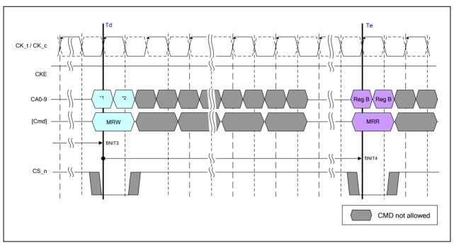
Figure 39 - Mode Register Write Timing for MRW RESET
