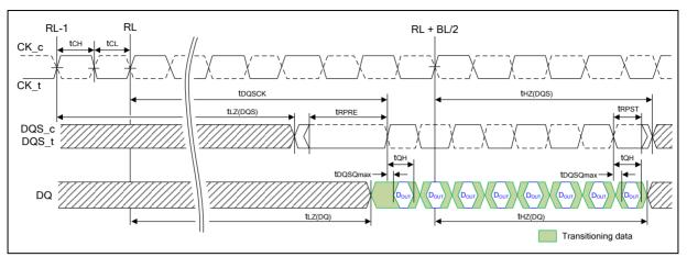
Figure 7 - Read Output Timing
