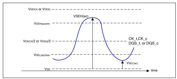
Figure 66 - Single-Ended Requirement for Differential Signals
