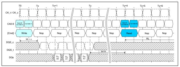
Figure 19 - Burst Write Followed By Burst Read
