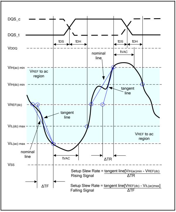
Figure 83 - Tangent line for setup time t<sub>DS</sub> for DQ with respect to strobe
