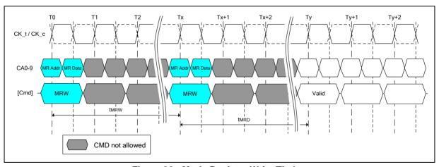
Figure 38 - Mode Register Write Timing
