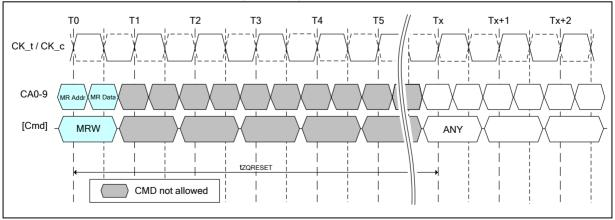
Figure 43 - ZQ Calibration Reset Timing
