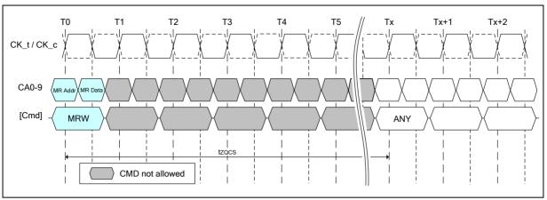
Figure 41 - ZQ Calibration Short Timing
