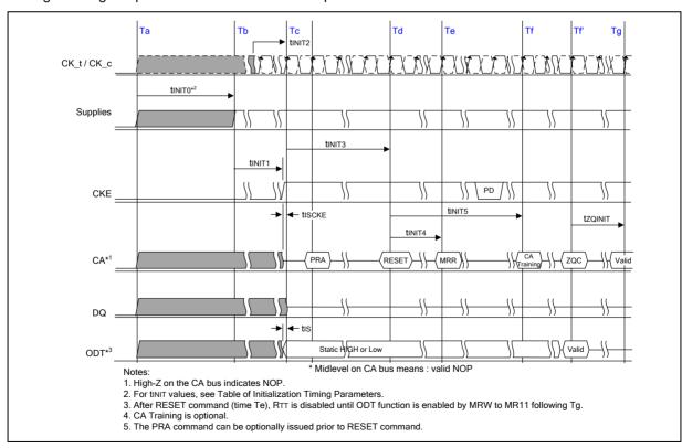
Figure 2: Voltage Ramp and Initialization Sequence
