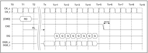
Figure 53 - Read to Power-Down Entry
