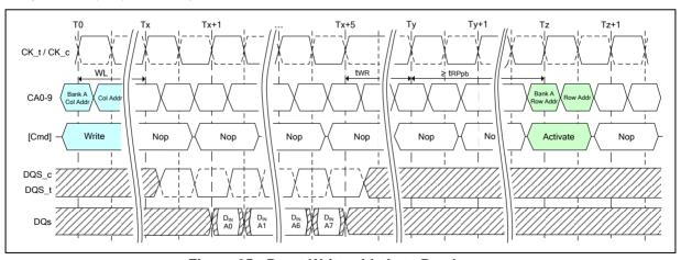
Figure 25 - Burst Write with Auto Precharge
