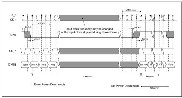
Figure 50 - Basic Power-Down Entry and Exit Timing
