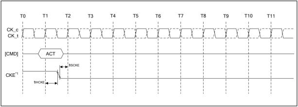
Figure 58 - Activate Command to Power-Down Entry
