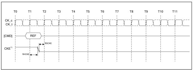
Figure 57 - Refresh Command to Power-Down Entry
