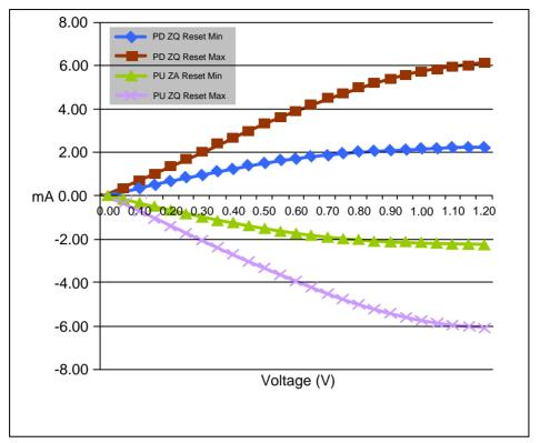
Figure 74 – I-V Curve after ZQ Reset
