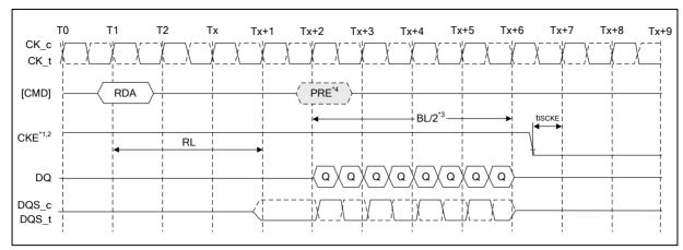
Figure 54 - Read with Auto Precharge to Power-Down Entry
