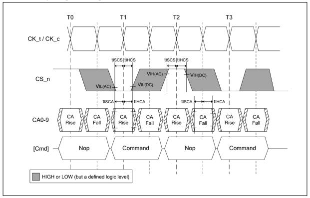
Figure 5 - Command Input Setup and Hold Timing
