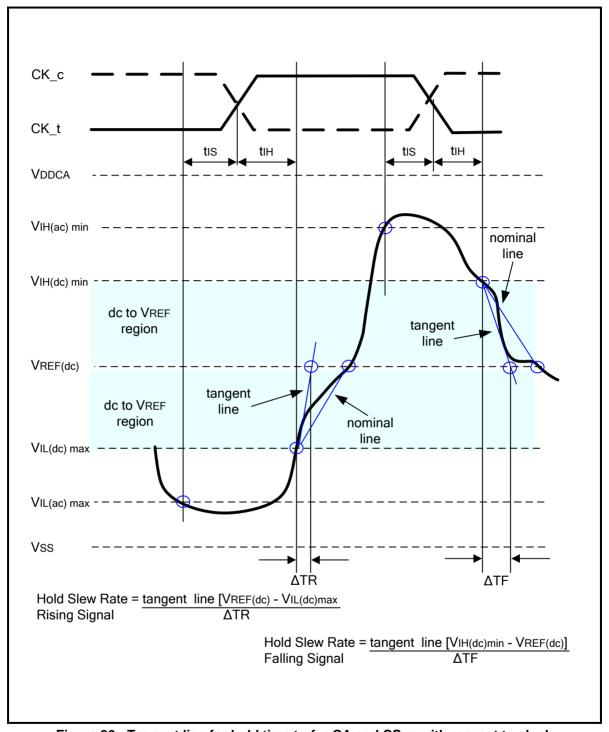
Figure 80 - Tangent line for hold time  $t_{\text{IH}}$  for CA and CS\_n with respect to clock
