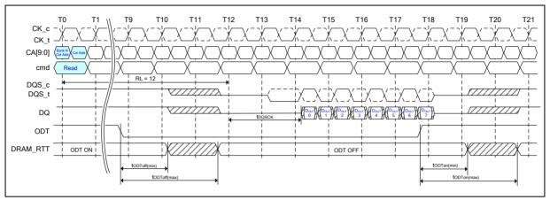
Figure 47 – Asynchronous ODT Timing Example for RL = 12
