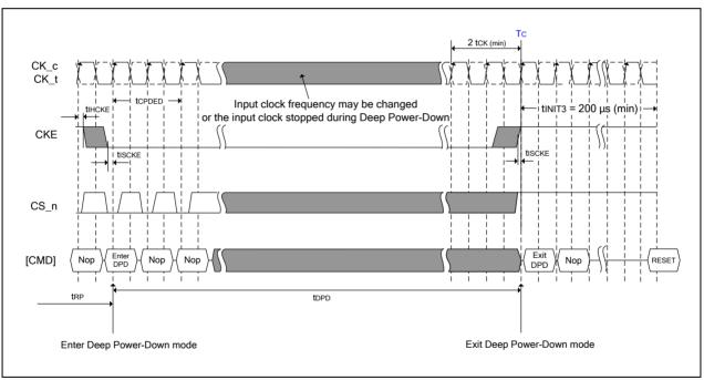
Figure 62 - Deep power down entry and exit timing diagram
