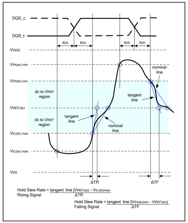
Figure 84 - Tangent line for hold time t<sub>DH</sub> for DQ with respect to strobe
