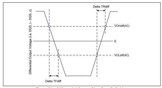
Figure 70 - Differential Output Slew Rate Definition
