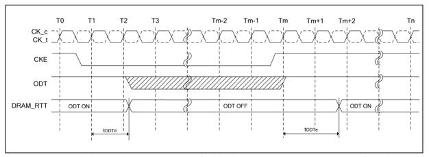
Figure 49 –ODT Timing During Power Down, Self Refresh, Deep Power Down Entry/Exit Example Notes:
