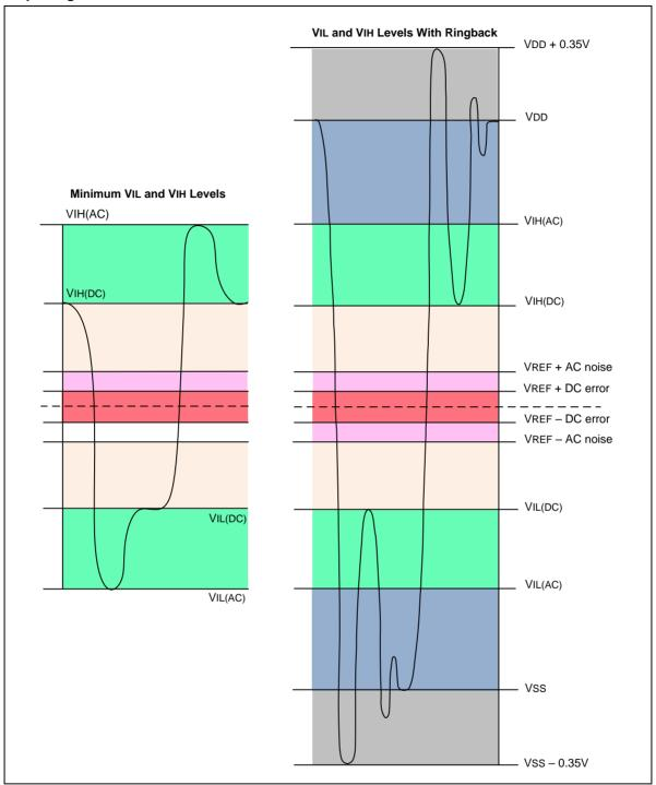
Figure 64 - LPDDR3 Input Signal
