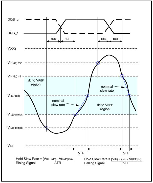
Figure 82 - Nominal slew rate for hold time t<sub>DH</sub> for DQ with respect to strobe
