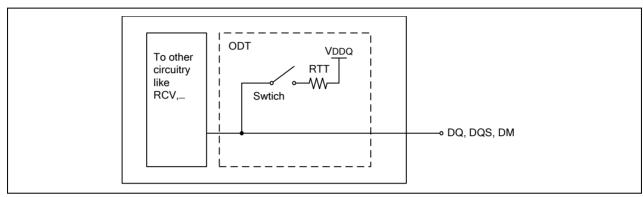
Figure 46 - Functional Representation of ODT
