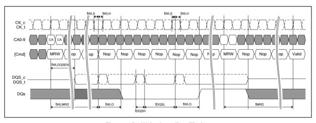
Figure 45 - Write Leveling Timing
