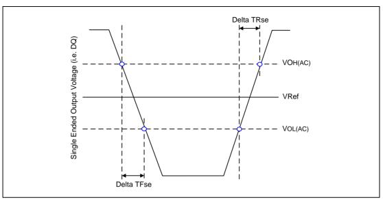
Figure 69 - Single Ended Output Slew Rate Definition
