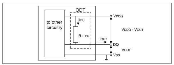
Figure 76 – Functional representation of On-Die Termination
