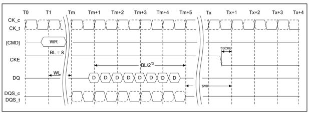
Figure 55 - Write to Power-Down Entry
