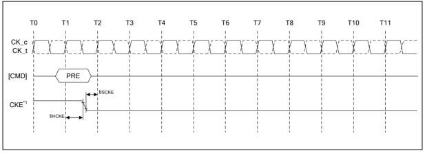
Figure 59 - Precharge Command to Power-Down Entry
