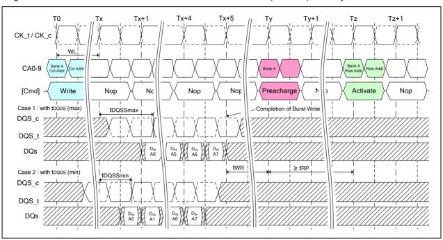
Figure 23 - Burst Write Followed by Precharge
