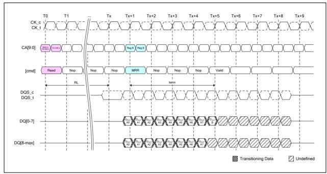
Figure 33 - Read to MRR Timing
