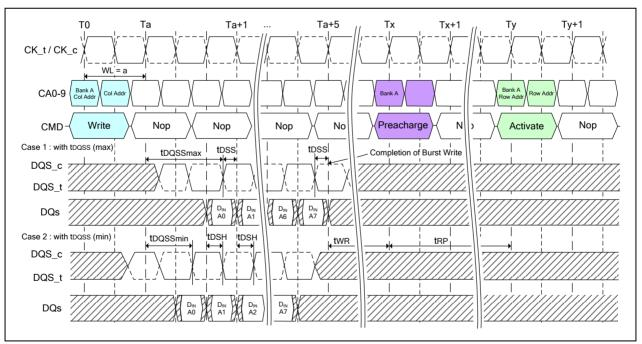
Figure 16 - Burst Write
