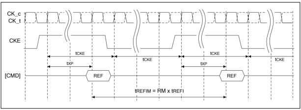
Figure 52 - Refresh-to-Refresh Timing in CKE-Intensive Environments
