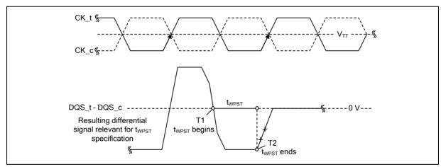
Figure 18 - Method for calculating twest Transitions and Endpoints
