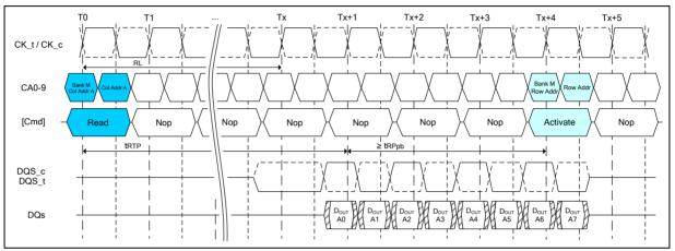
Figure 24 - Burst Read with Auto Precharge
