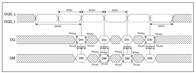
Figure 15 - Data input (write) timing
