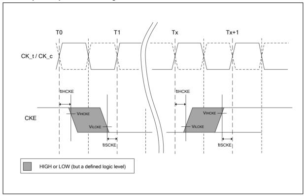
Figure 6 - CKE Input Setup and Hold Timing
