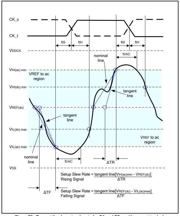
Figure 79 - Tangent line for setup time  $t_{\text{IS}}$  for CA and CS\_n with respect to clock
