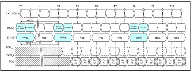
Figure 20 - Seamless burst write: WL = 4, tCCD = 4
