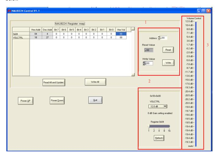
The first step is to hit the Power Up button. This will ensure any changes in the register settings are written to the register map of the chip.
