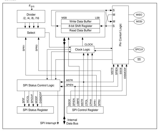
Figure 6.12-1 SPI Block Diagram
