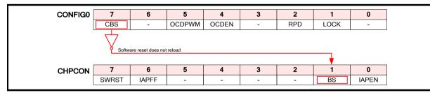
Figure 6.2-1 CONFIG0 Any Reset Reloading
