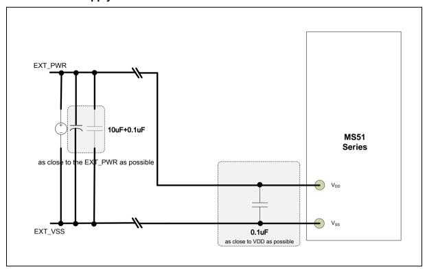
Figure 7.1-1 Numara® MS51 Power Supply Circuit
