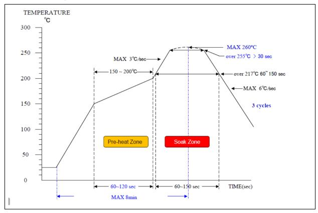
Figure 8.6-1 Soldering profile from J-STD-020C
