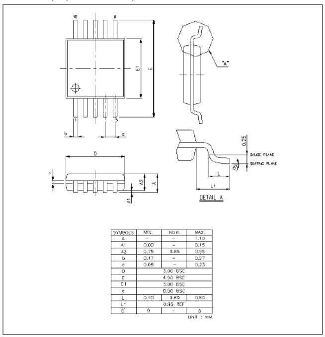
Figure 9.2-1 MSOP -10 Package Dimension
