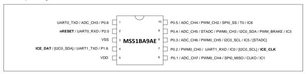
Figure 4.1-2 Pin Assignment of MSOP-10 Package
