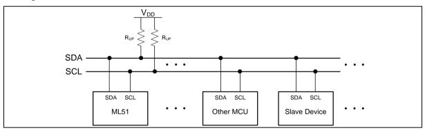
Figure 6.11-1 I<sup>2</sup>C Bus Interconnection
