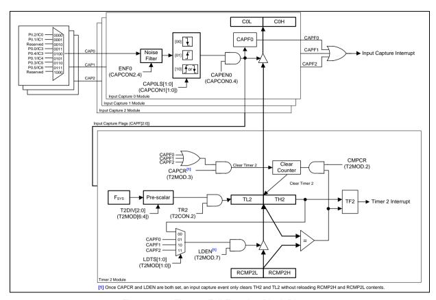
Figure 6.6-1 Timer 2 Full Function Block Diagram
