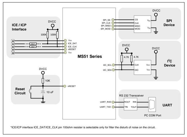
Figure 7.2-1 NuMicro® MS51 Peripheral Interface Circuit
