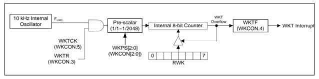
Figure 6.8-1 Self Wake-Up Timer Block Diagram
