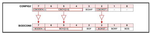
Figure 6.2-2 CONFIG2 Power-On Reset Reloading
