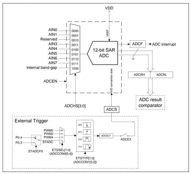
Figure 6.13-112-bit ADC Block Diagram
