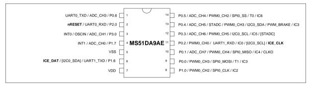
Figure 4.1-1 Pin Assignment of TSSOP-14 Package
