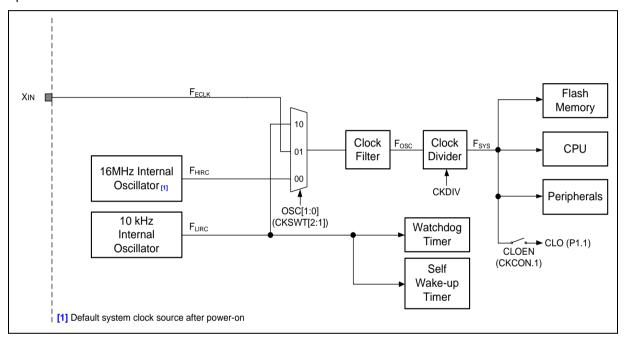
Figure 6.3-1 Clock System Block Diagram
