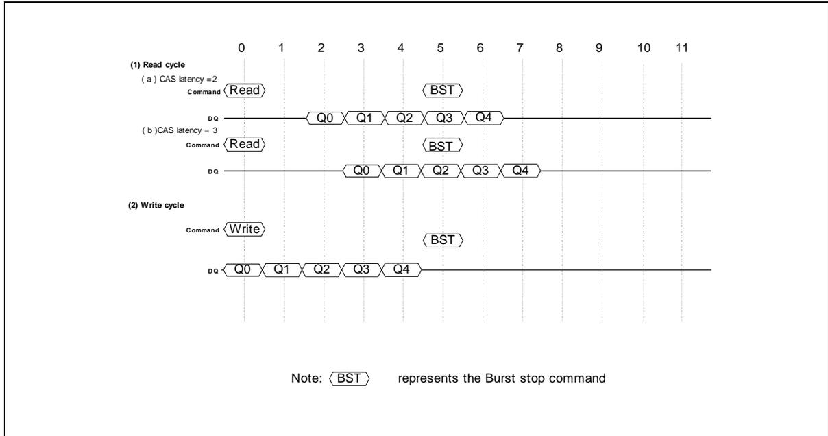
11.22 Timing Chart of Burst Stop Cycle (Precharge Command)
