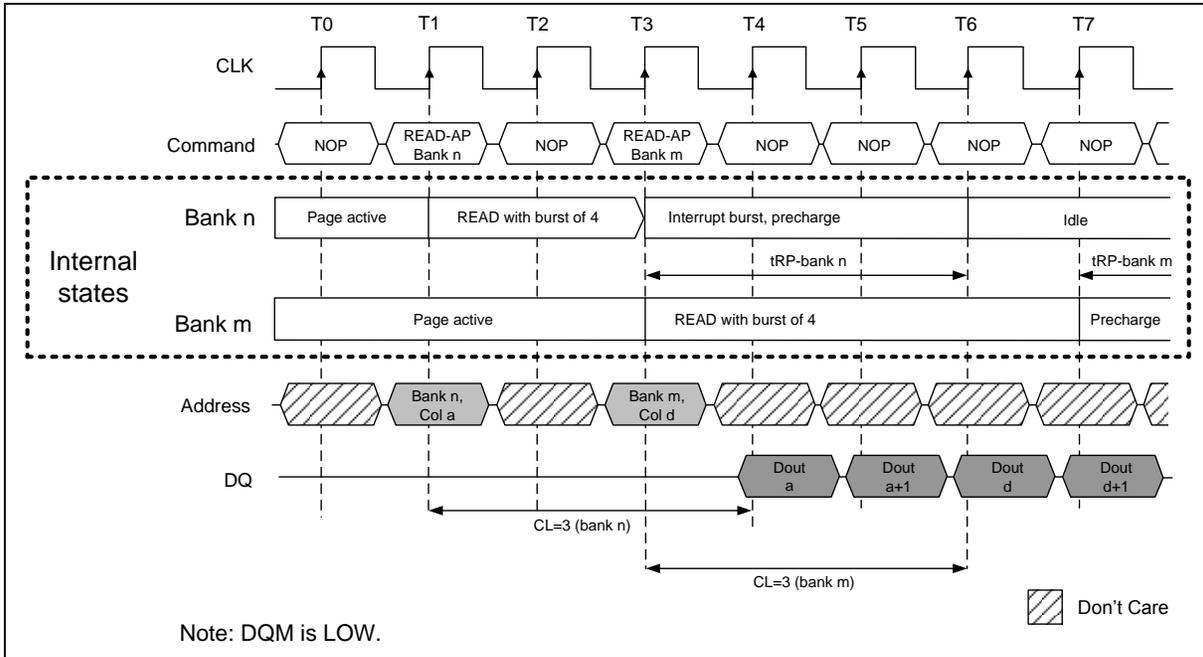
**8.3.3 READ with auto precharge interrupted by a WRITE (with or without auto precharge)**
