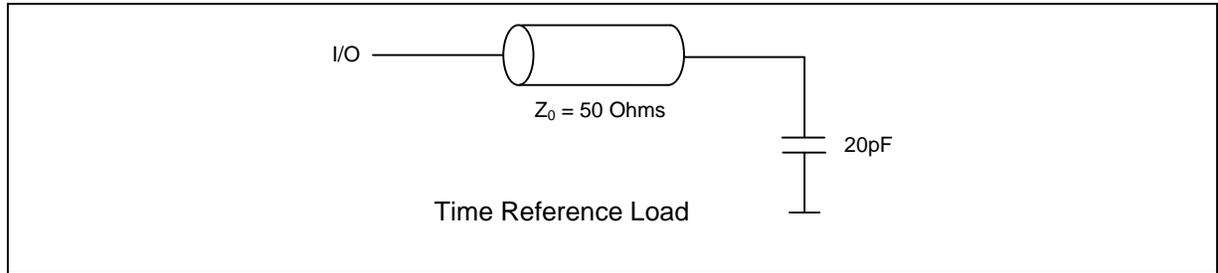
Input signal transition time between V<sub>IH</sub> and V<sub>IL</sub> is assumed as 1 Volts/nS.
