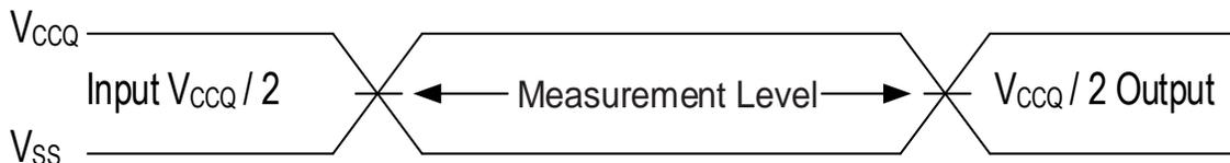
Figure 21 - Input Waveforms and Measurement Levels
