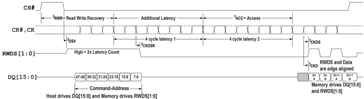
**Figure 23 - Read Timing Diagram — With Additional Latency**
