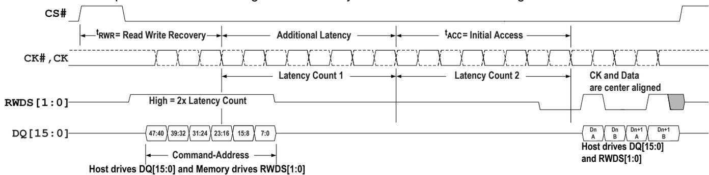
**Figure 7 - Write Transaction with Additional Initial Latency**
