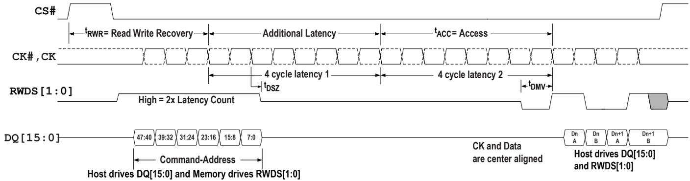
**Figure 25 - Write Timing Diagram — With Additional Latency**
