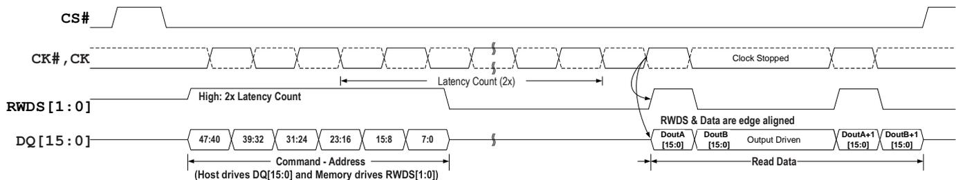
Figure 9 - Active Clock Stop during Read Transaction (DDR)
