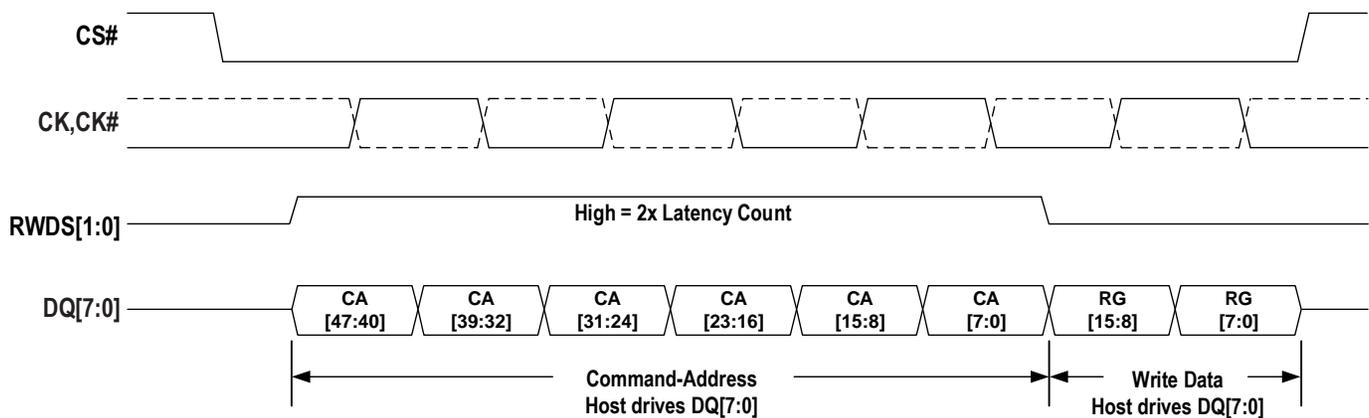
**Figure 8 - Write Operation without Initial Latency (Register Write)**
