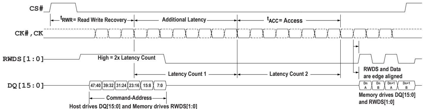
**Figure 6 - Read Transaction with Additional Initial Latency**
