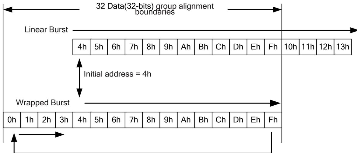
**Figure 2 - Linear Versus Wrapped Burst Sequence**
