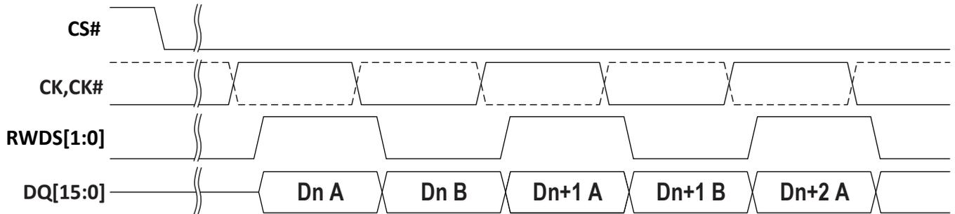
Figure 4 - Data Placement during a Read Transaction
