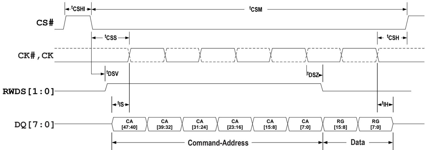
Figure 26 - Write Operation without Initial Latency (Register Write)
