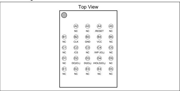
Figure 1d. W25Q64JW Ball Assignments, 24-ball TFBGA 8x6-mm (Package Code TB)
