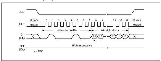
Figure 45. Erase Security Registers Instruction (SPI Mode only)
