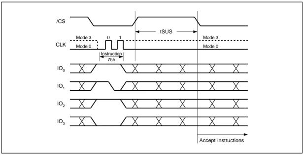
Figure 35b. Erase/Program Suspend Instruction (QPI Mode)
