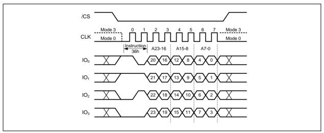
Figure 53b. Individual Block/Sector Lock Instruction (QPI Mode)
