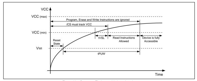
Figure 58a. Power-up Timing and Voltage Levels
