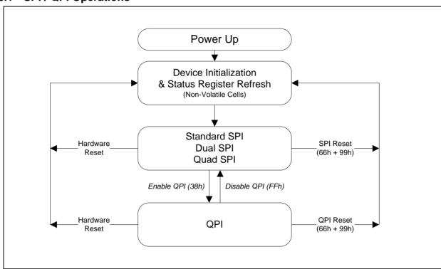
Figure 3, W25Q64JV Serial Flash Memory Operation Diagram
