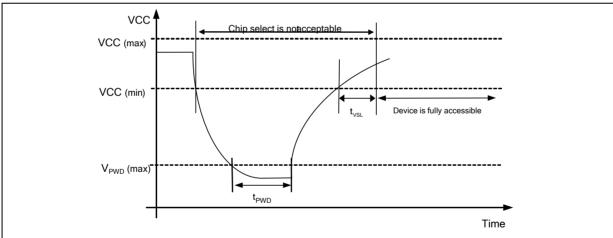
Figure 58c. Power Cycle Requirement
