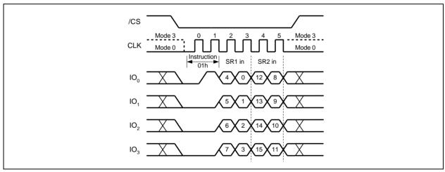
Figure 9d. Write Status Register-1/2 Instruction (QPI Mode)
