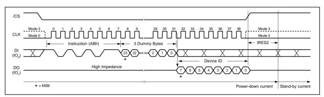
Figure 38c. Release Power-down / Device ID Instruction (SPI Mode)
