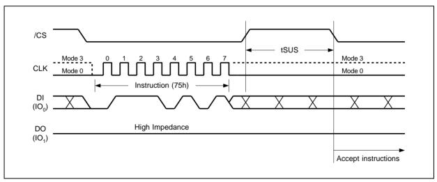
Figure 35a. Erase/Program Suspend Instruction (SPI Mode)
