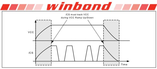
Figure 58b. Power-up, Power-Down Requirement
