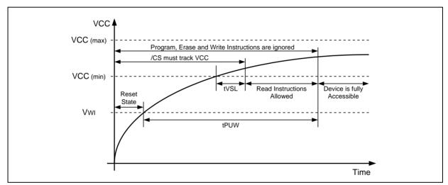
Figure 58a. Power-up Timing and Voltage Levels
