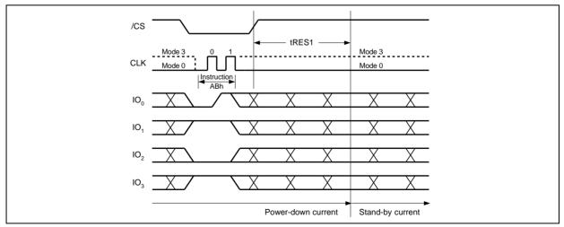
Figure 38b. Release Power-down Instruction (QPI Mode)
