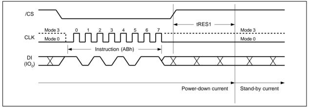
Figure 38a. Release Power-down Instruction (SPI Mode)
