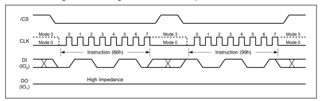
Figure 58a. Enable Reset and Reset Instruction Sequence (SPI Mode)
