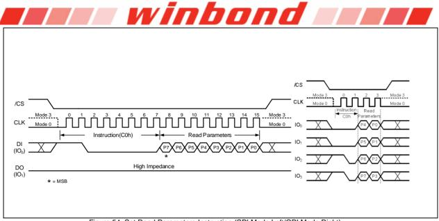
Figure 54. Set Read Parameters Instruction (SPI Mode Left/QPI Mode Right)
