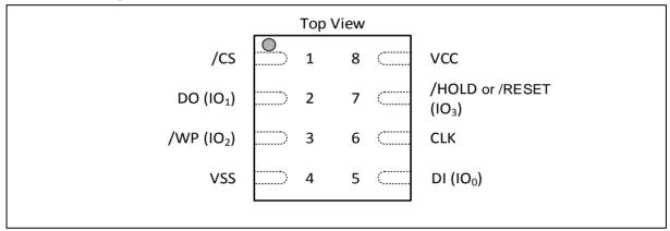
Figure 1b. W25Q16RV Pad Assignments, 8-pad WSON 6x5-mm, USON 2X3-mm (Package Code ZP, XH)
