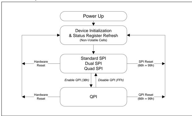
Figure 3. W25Q16RV Serial Flash Memory Operation Diagram
