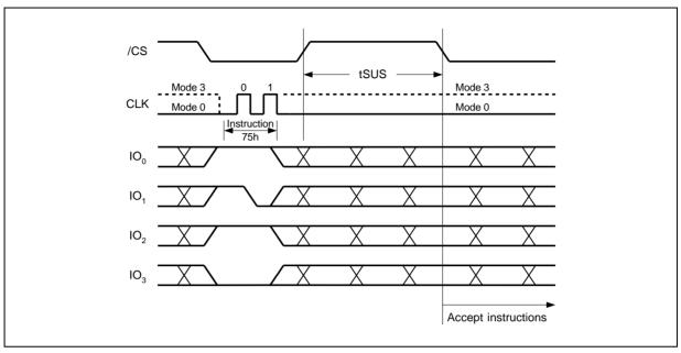
Figure 35b. Erase/Program Suspend Instruction (QPI Mode)
