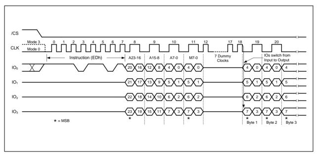
Figure 27a. DTR Fast Read Quad I/O (Initial instruction or previous M5-4≠10, SPI Mode)
