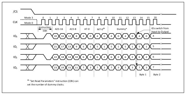
Figure 24c. Fast Read Quad I/O Instruction (Initial Instruction or previous M5-4≠10, QPI Mode)
