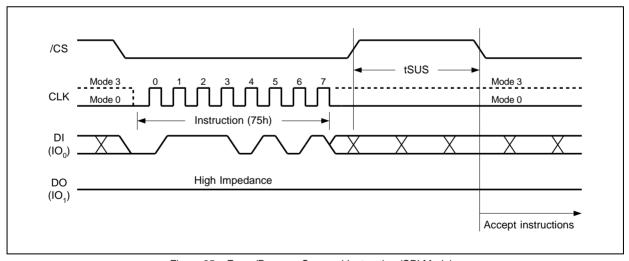
Figure 35a. Erase/Program Suspend Instruction (SPI Mode)
