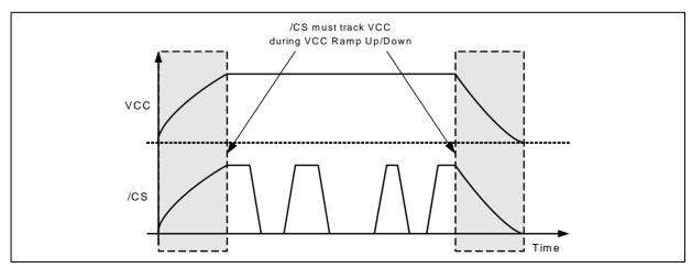
Figure 58b. Power-up, Power-Down Requirement
