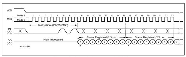
Figure 8a. Read Status Register Instruction (SPI Mode)
