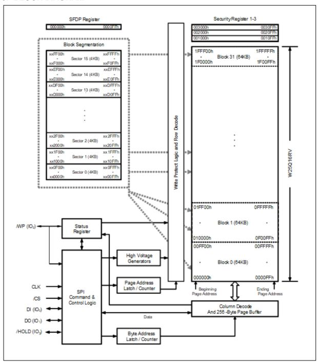
Figure 2. W25Q16RV Serial Flash Memory Block Diagram
