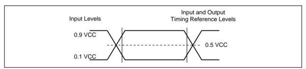
Figure 59. AC Measurement I/O Waveform
