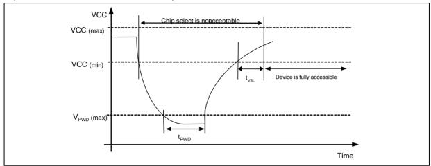
Figure 58c. Power Cycle Requirement
