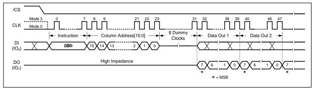
Figure 8-23 Fast Read Instruction (Buffer Read Mode, BUF=1)
