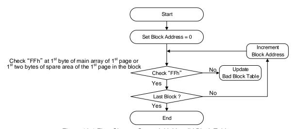
Figure 10-1 Flow Chart to Create Initial Invalid Block Table
