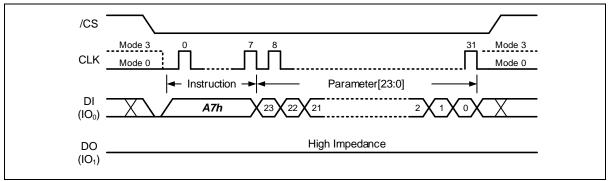
Figure 8-12 Built-in ECC Decode Check Instruction
