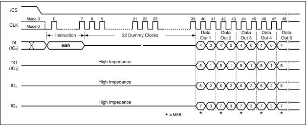
Figure 8-28 Fast Read Quad Output Instruction (Continuous Read Mode or Sequential Read Mode, BUF=0)
