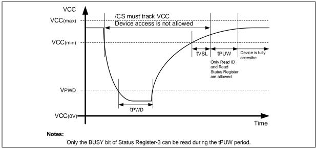
Figure 9-1 Power-up Timing and Voltage Levels
