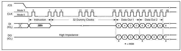
Figure 8-26 Fast Read Dual Output Instruction (Continuous Read Mode or Sequential Read Mode, BUF=0)
