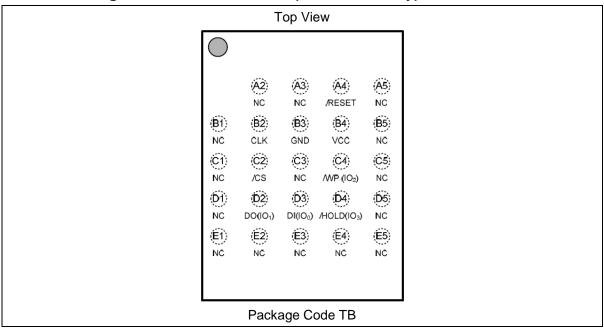
Figure 3-2 W25NxxLW Ball Assignments, 24-ball TFBGA 8x6-mm (Package Code TB)
