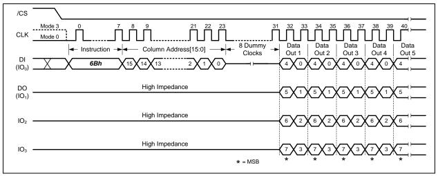
Figure 8-27 Fast Read Quad Output Instruction (Buffer Read Mode, BUF=1)
