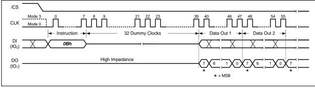
Figure 8-24 Fast Read Instruction (Continuous Read Mode or Sequential Read Mode, BUF=0)
