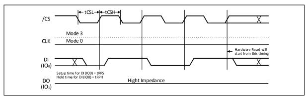
Figure 6-2 Reset Signaling Protocol
