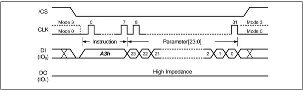
Figure 8-11 Built-in ECC Encode Check Instruction
