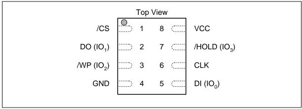
Figure 3-1 W25NxxLW Pad Assignments, 8-pad WSON 8x6-mm (Package Code ZE)
