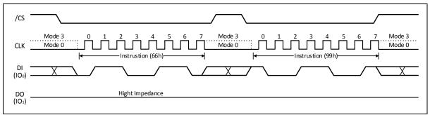
Figure 8-2 Device Reset Instruction (66h+99h)
