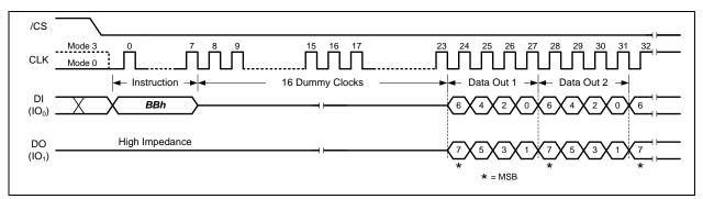
Figure 8-30 Fast Read Dual I/O Instruction (Continuous Read Mode or Sequential Read Mode, BUF=0)
