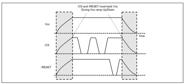
Figure 9-2 Power-up, Power-down Requirement
