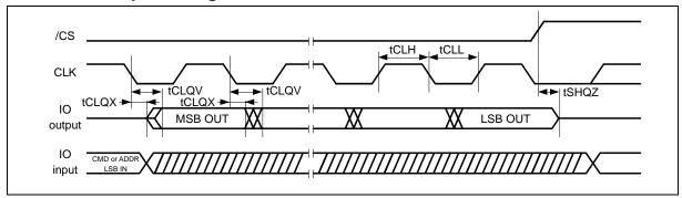
Figure 9-4 Serial Output Timing
