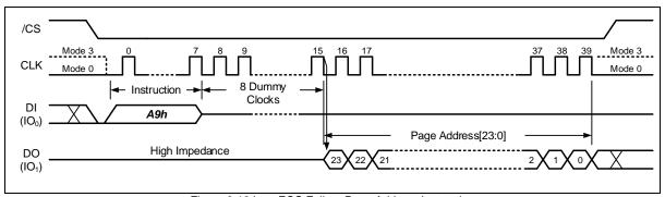
Figure 8-10 Last ECC Failure Page Address Instruction
