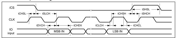
Figure 9-5 Serial Input Timing
