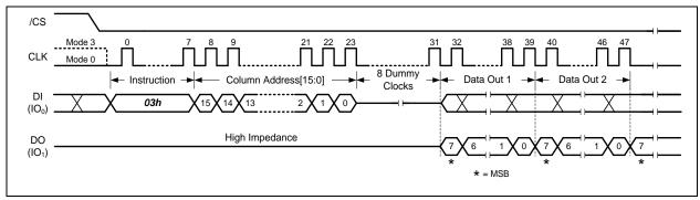
Figure 8-21 Read Data Instruction (Buffer Read Mode, BUF=1)
