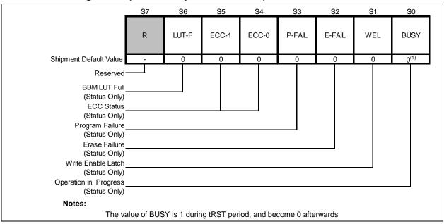
Figure 7-3 Status Register-3 (Address Cxh)
