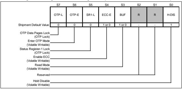
Figure 7-2 Configuration Register / Status Register-2 (Address Bxh)
