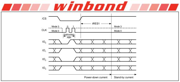
Figure 38b. Release Power-down Instruction (QPI Mode)
