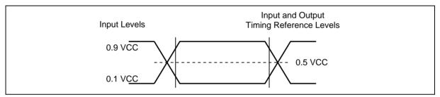
Figure 59. AC Measurement I/O Waveform
