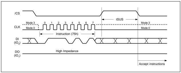
Figure 35a. Erase/Program Suspend Instruction (SPI Mode)
