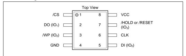
Figure 1a. W25Q32FV Pin Assignments, 8-pin SOIC / VSOP 208-mil (Package Code SS / ST)
