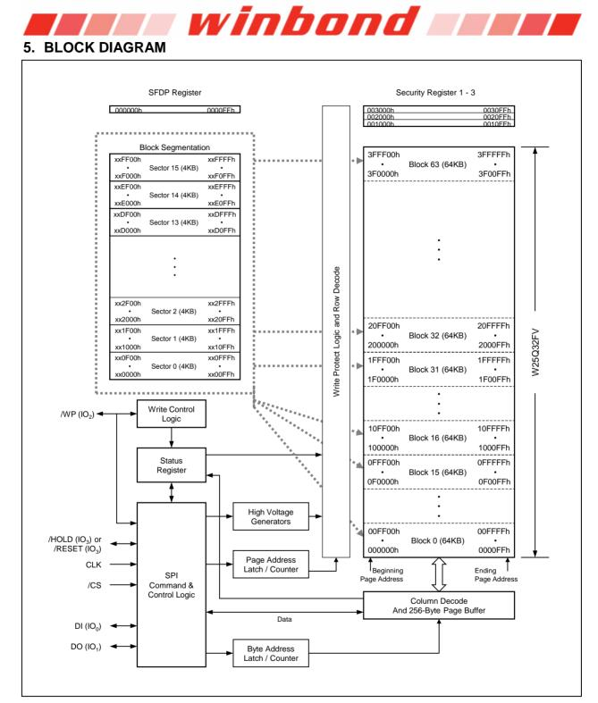
Figure 2. W25Q32FV Serial Flash Memory Block Diagram
