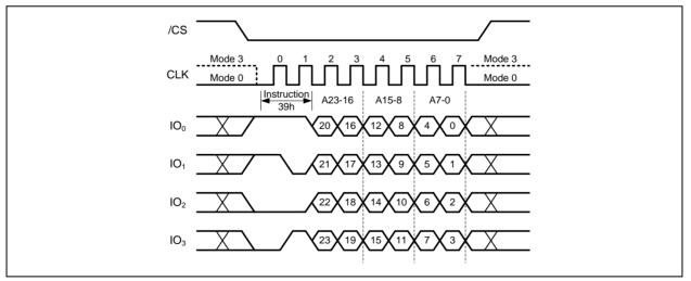
Figure 53b. Individual Block Unlock Instruction (QPI Mode)
