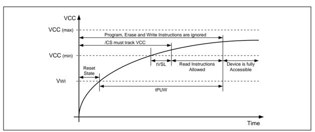
Figure 58a. Power-up Timing and Voltage Levels
