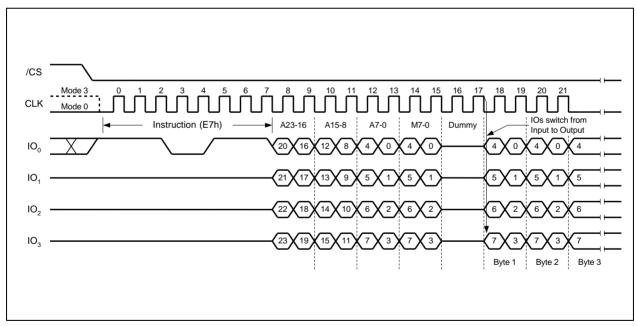
Figure 26a. Word Read Quad I/O Instruction (Initial instruction or previous M5-4 ≠ 10, SPI Mode only)
