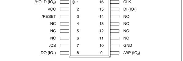
Figure 1c. W25Q32FV Pin Assignments, 16-pin SOIC 300-mil (Package Code SF)
