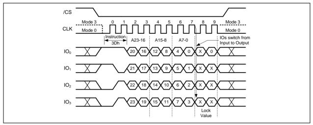
Figure 54b. Read Block Lock Instruction (QPI Mode)
