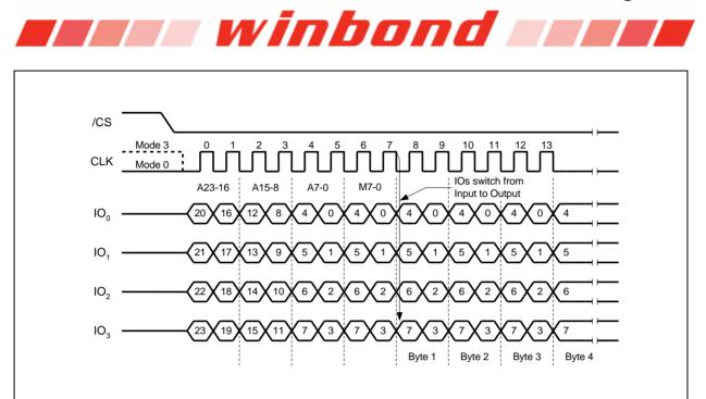
Figure 27b. Octal Word Read Quad I/O Instruction (Previous instruction set M5-4 = 10, SPI Mode only)
