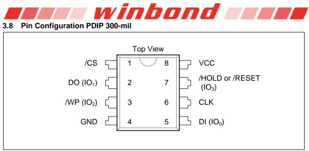
Figure 1e. W25Q32FV Pin Assignments, 8-pin PDIP (Package Code DA)
