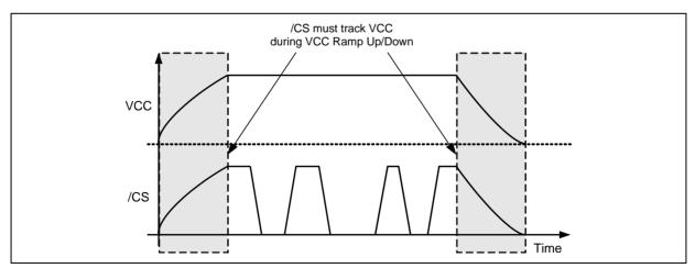
Figure 58b. Power-up, Power-Down Requirement
