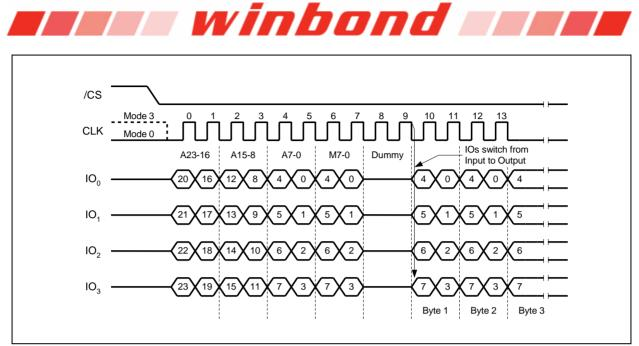
Figure 26b. Word Read Quad I/O Instruction (Previous instruction set M5-4 = 10, SPI Mode only)
