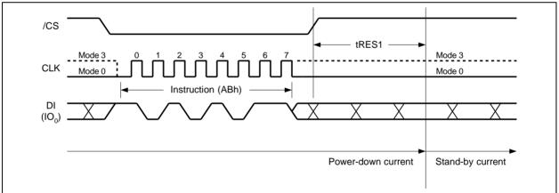
Figure 38a. Release Power-down Instruction (SPI Mode)
