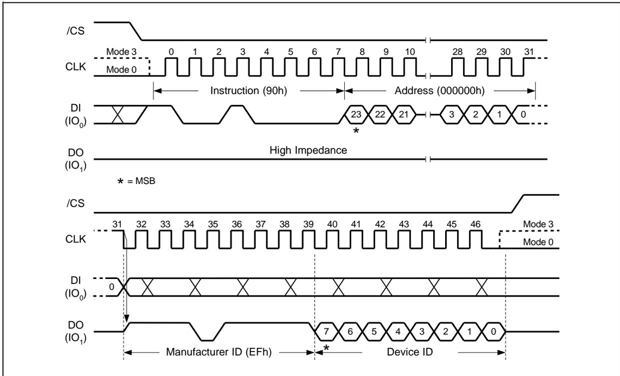
Figure 46. Read Manufacturer / Device ID Instruction (SPI Mode)
