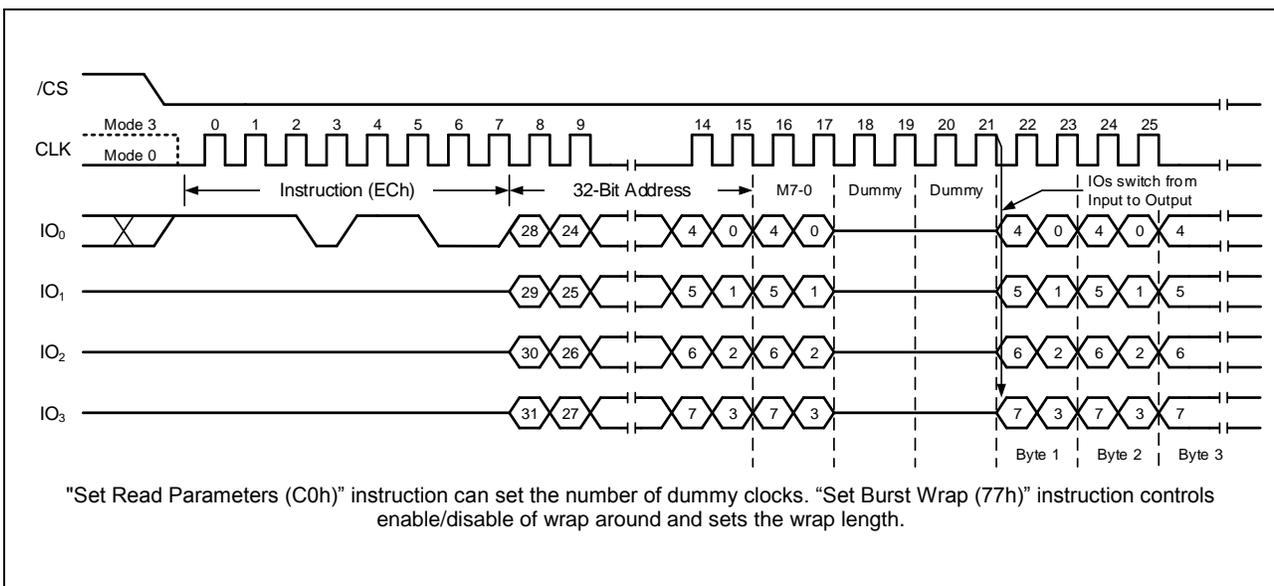
Figure 28a. Fast Read Quad I/O w/ 4-Byte Addr. (Initial instruction or previous M5-4=F<sub>x</sub>h, SPI Mode only)
