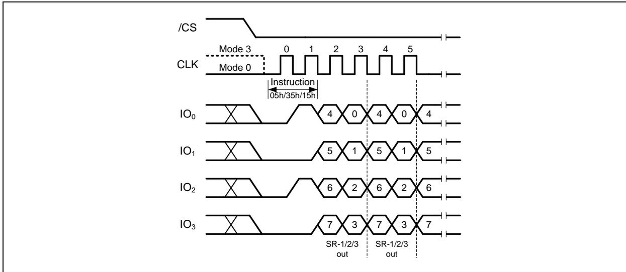
Figure 8b. Read Status Register Instruction (QPI Mode)
