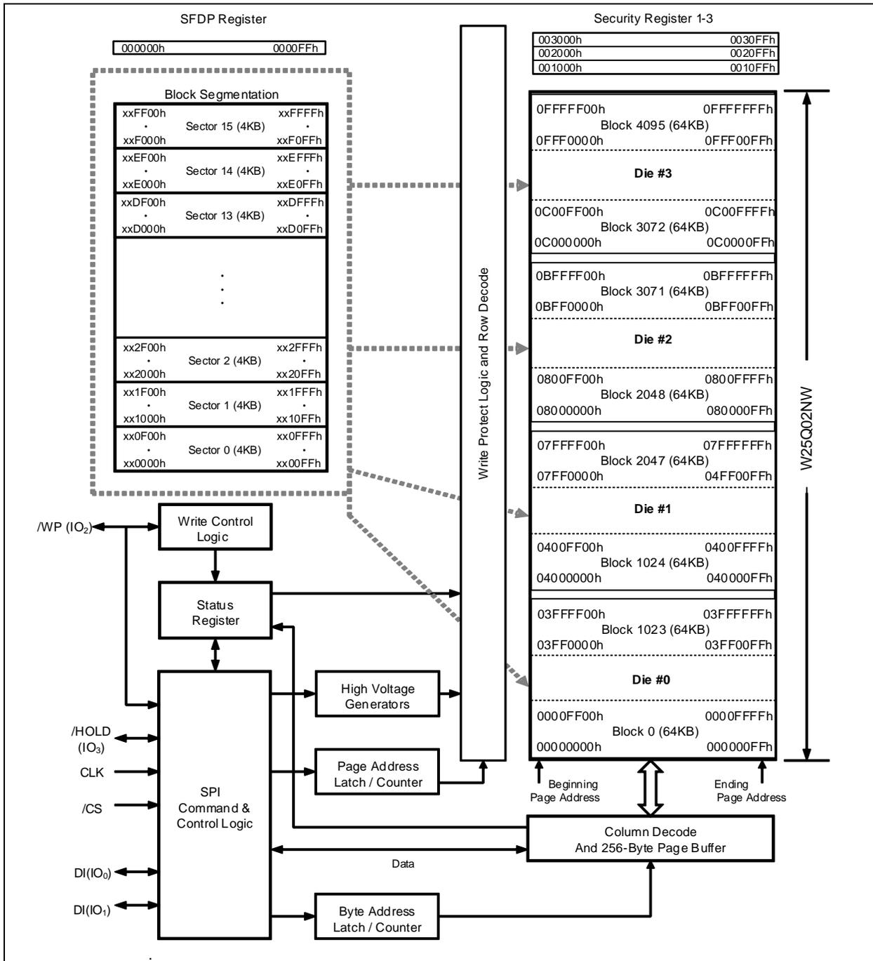
Figure 2. W25Q02NW Serial Flash Memory Block Diagram
