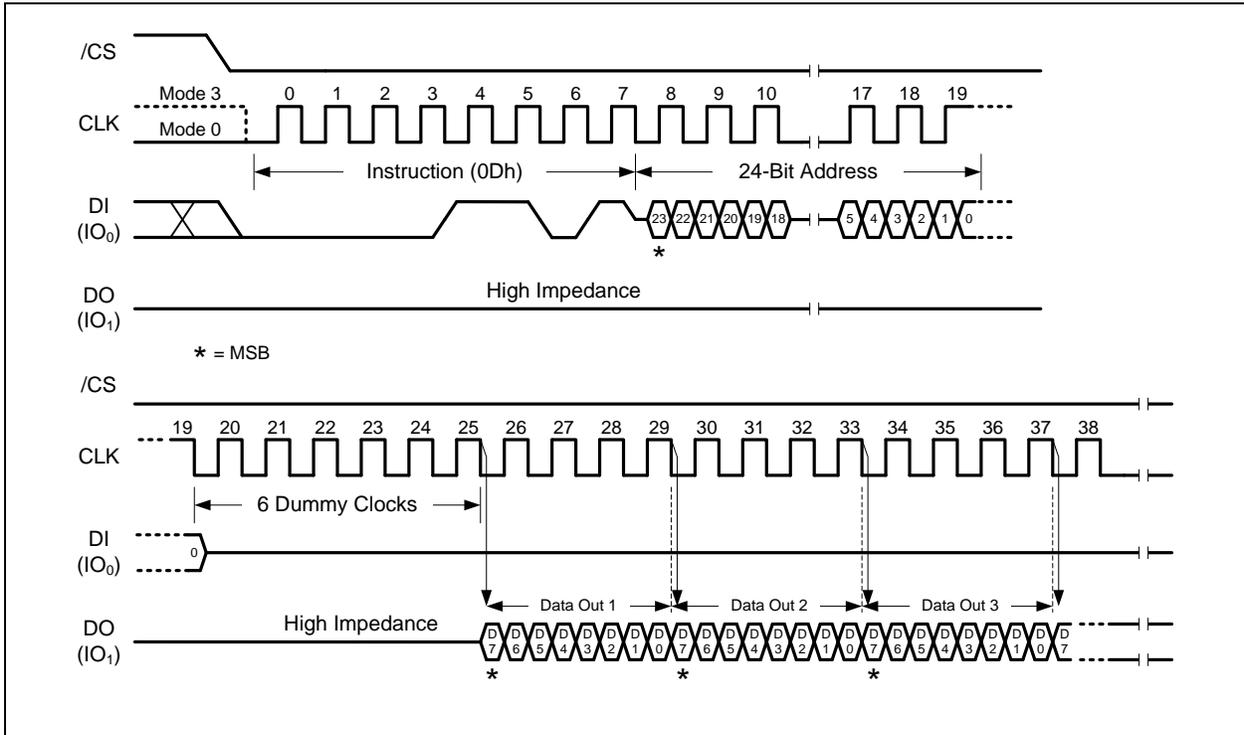
Figure 17a. DTR Fast Read Instruction (SPI Mode)
