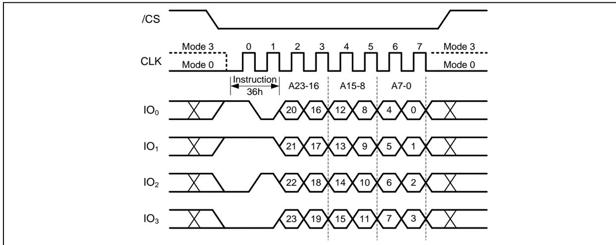
Figure 59b. Individual Block/Sector Lock Instruction (QPI Mode)
