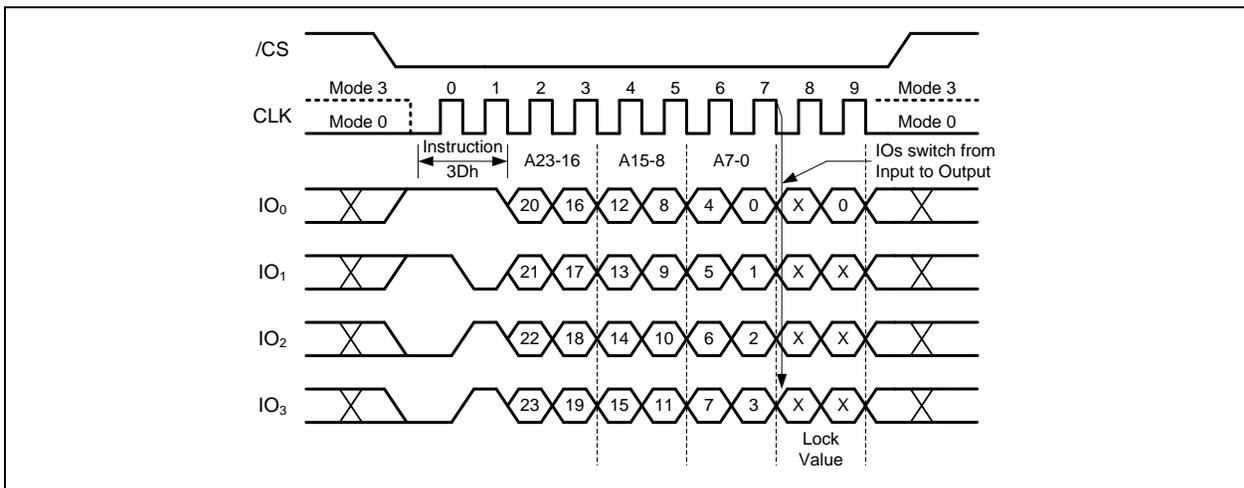
Figure 61b. Read Block Lock Instruction (QPI Mode)
