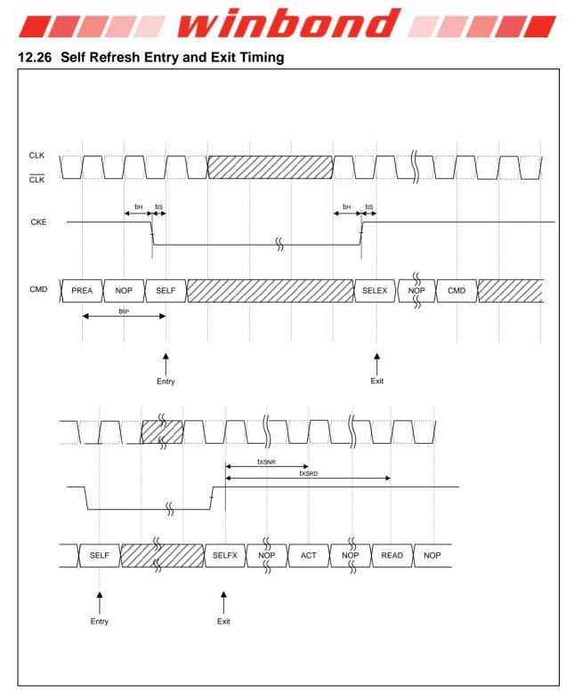
Note: If the clock frequency is changed during self refresh mode, a DLL reset is required upon exit.
