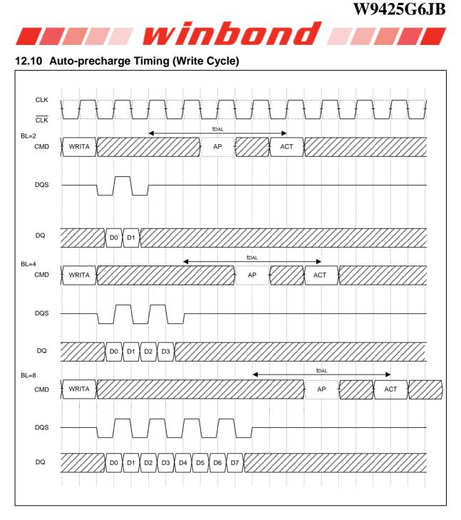
The Write with Auto-precharge command cannot be interrupted by any other command.
