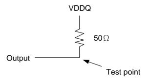
Figure 2: Pulldown slew rate test load
