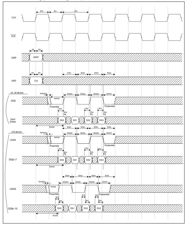
Note: x16 has two DQSs (UDQS for upper byte and LDQS for lower byte). Even if one of the 2 bytes is not used, both UDQS and LDQS must be toggled.
