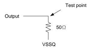
Figure 1: Pullup slew rate test load
