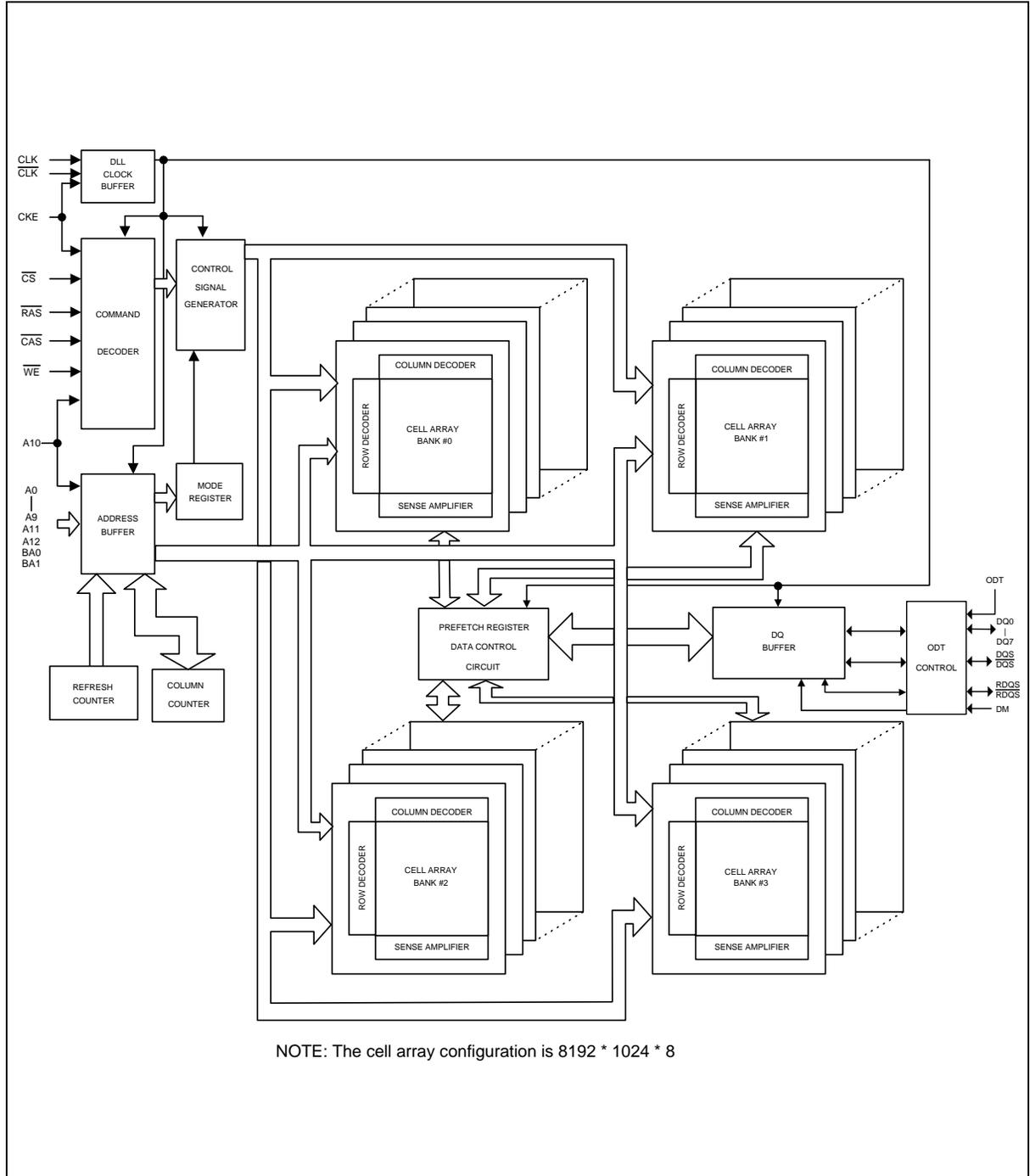
NOTE: The cell array configuration is 8192 \* 1024 \* 8
