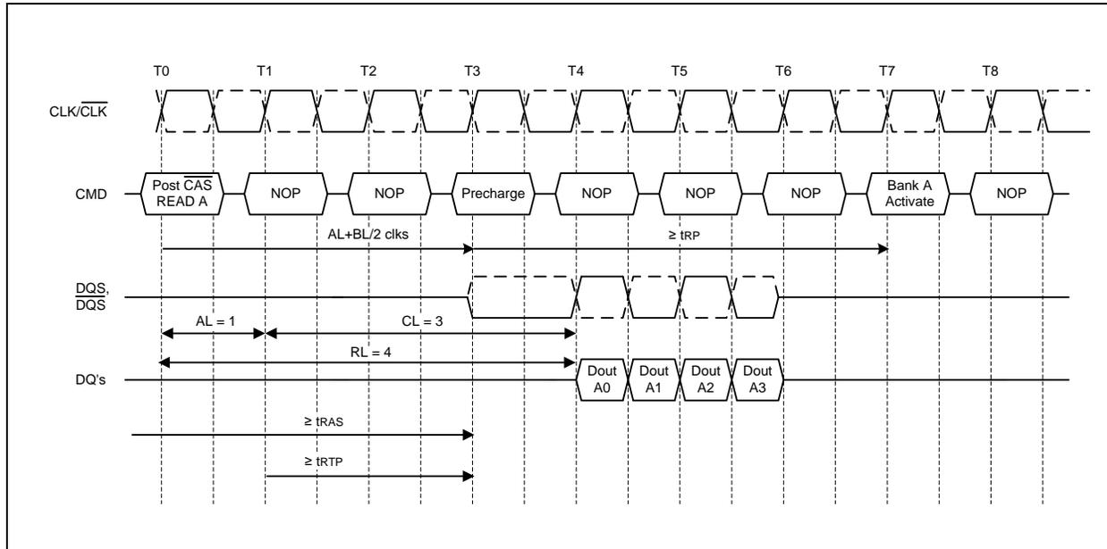
**11.16 Burst read operation followed by precharge: RL=4 (AL=1, CL=3, BL=8,  $t_{RTP} \leq 2\text{clks}$ )**
