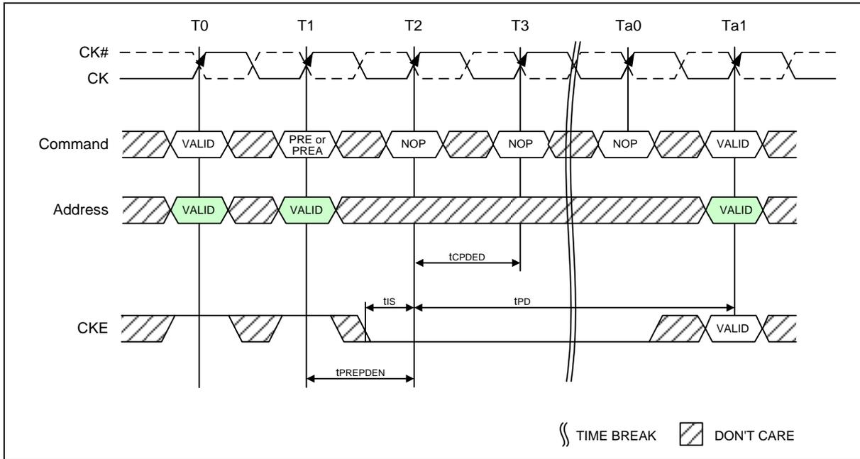
Figure 67 – Precharge / Precharge all Command to Power-Down Entry
