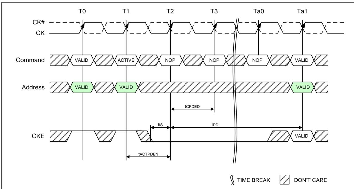
Figure 66 – Active Command to Power-Down Entry
