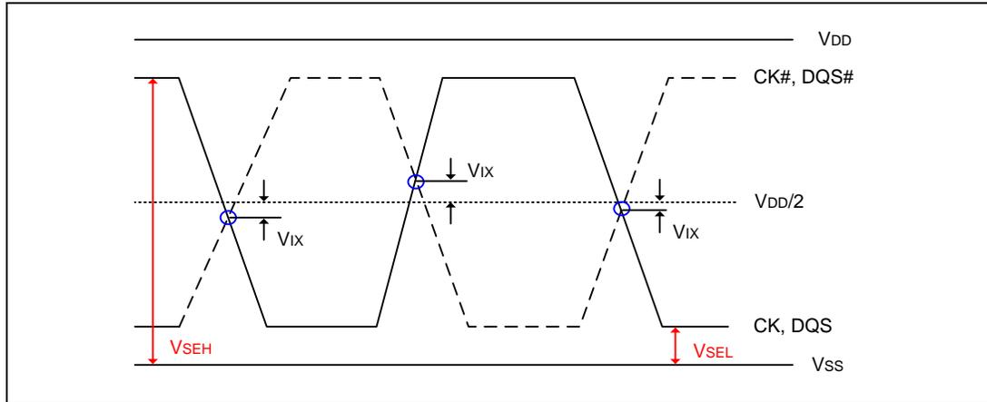
Figure 92 –  $V_{IX}$  Definition
