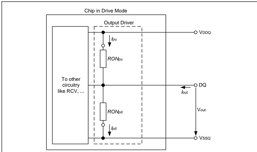
Figure 96 – Output Driver: Definition of Voltages and Currents
