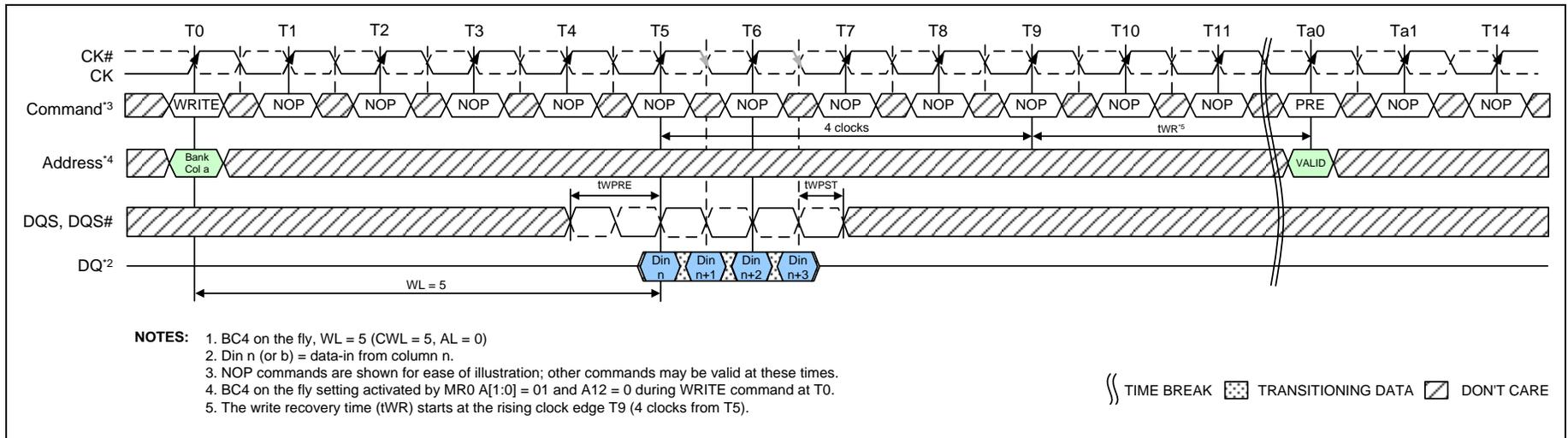
Figure 47 – WRITE (BC4) OTF to PRECHARGE Operation
