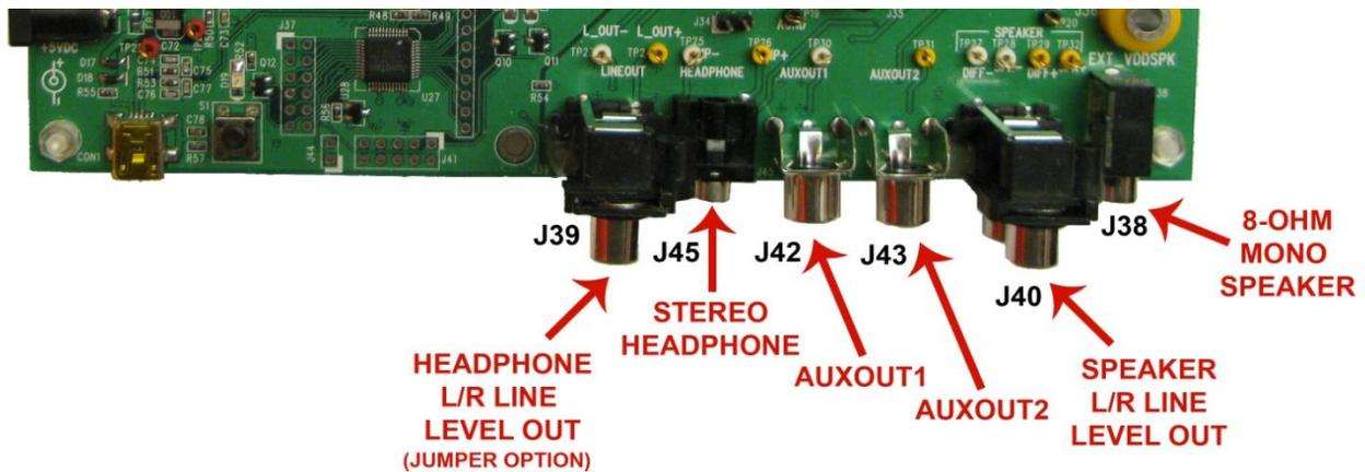
Figure 26: ANALOG OUTPUTS
