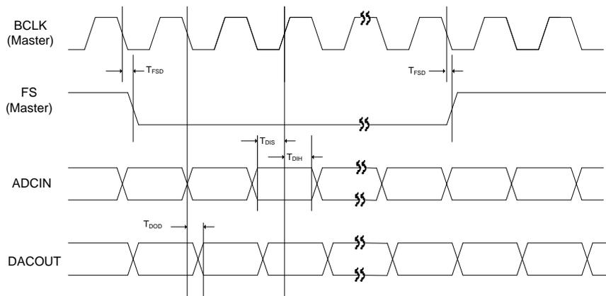
Figure 32: Digital Audio Interface Master Mode Timing
