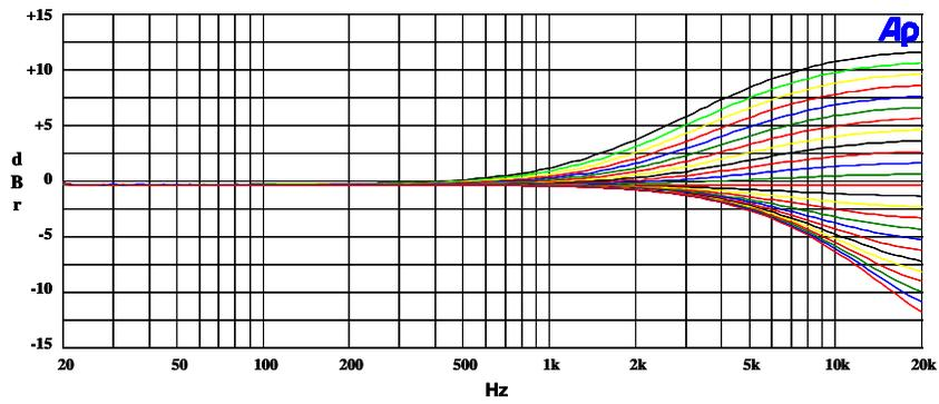
Figure 48: EQ Band 5 Gains for Lowest Cut-Off Frequency
