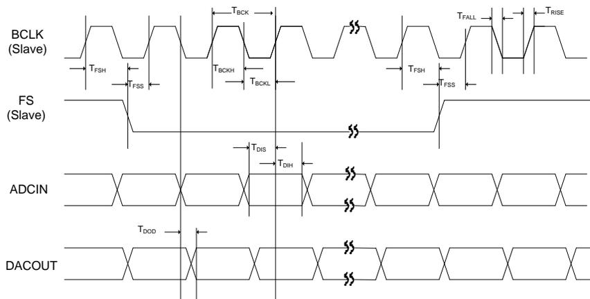
Figure 31: Digital Audio Interface Slave Mode Timing
