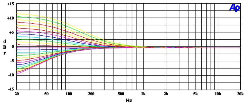
Figure 41: EQ Band 1 Gains for Lowest Cut-Off Frequency
