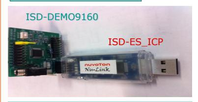
Demonstration board. Connects directly to the ISD-ES\_ICP\_USB programmer for custom programming of on board ISD9160 IC. The Demo Contains all necessary signals to be used as prototype board in customer's application Sytem..
