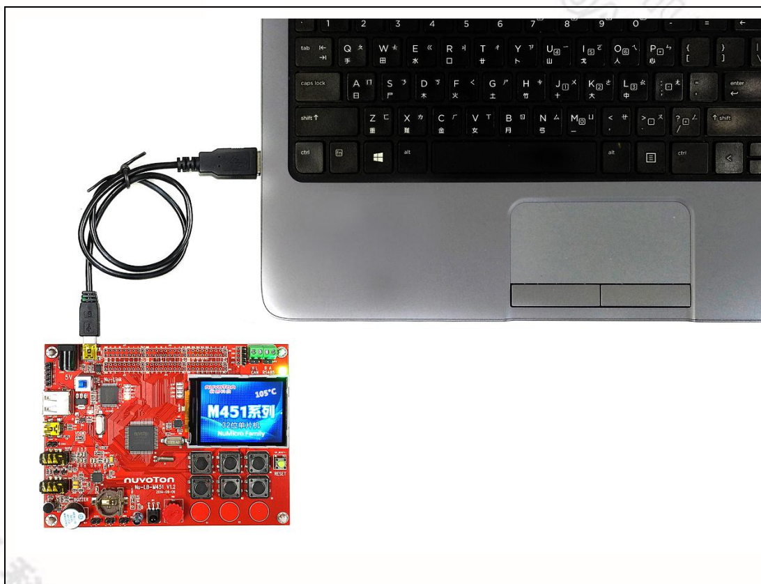
Figure 3-1 Nu-LB-M451 Hardware Setup
