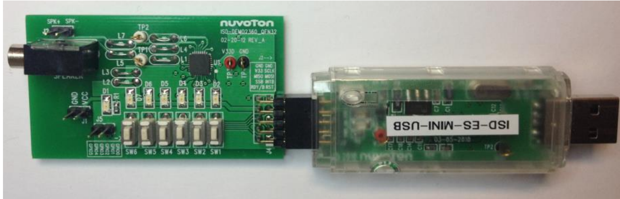
Picture 3.2-1 Demo board connects to USB dongle board with both boards facing up
