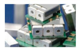
Applying the ceramic technology that has been accumulated over many years, MARUWA has developed high-performance band pass filters. The use of our original dielectric coaxial resonator permits production of custom-made products that will meet customers' needs.
